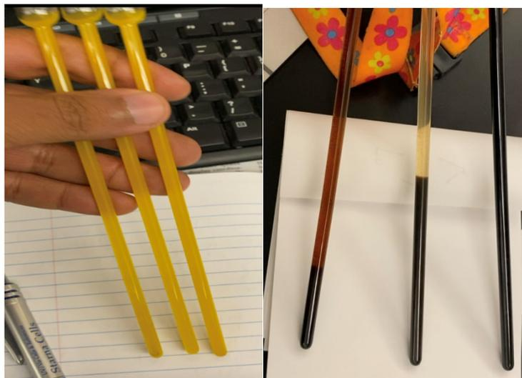
**Figure S10.** Pictures of NMR tubes from reduction of **2** with 1, 2 and 4 equivalents of KCs respectively.
