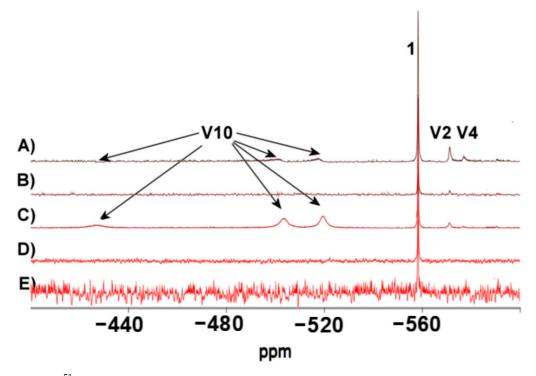
**Figure 7.** <sup>51</sup>V NMR spectra DMSO-*d*<sub>6</sub>:D<sub>2</sub>O (1:9) solutions of (**A**) 1.00 mM of **1** + 1.00 mM NaVO<sub>3</sub>, pD = 5.9 (**B**) 1.00 mM of **1** pD = 5.9 (**C**) 1.00 mM of **1** + 1.00 mM NaVO<sub>3</sub>, pD = 5.0 (**D**) 1.00 mM of **1**, pD = 5.0. (**E**) 0.10 mM of **1**, pD = 7.0. V10, V2, V4 are the vanadium oligomers.
