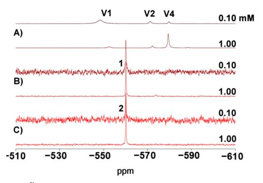
**Figure 6.** <sup>51</sup>V NMR spectra DMSO- $d_6$ :D<sub>2</sub>O (1:9) solutions of (**A**) NaVO<sub>3</sub>, (**B**) **1**, (**C**) **2** at pD ~ 7. V1, V2, V4 are the vanadium oligomers.
