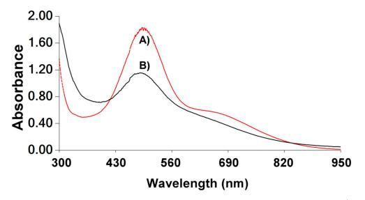
**Figure 4.** UV-vis spectra of CHCl<sub>3</sub> solutions of 0.500 mM of (**A**) **1m** [ $\lambda(\varepsilon) = 493$  nm (3600 M<sup>-1</sup>cm<sup>-1</sup>), 682 nm (1140 M<sup>-1</sup> cm<sup>-1</sup>)] and (**B**) **2m** [ $\lambda(\varepsilon) = 484$  nm (2300 M<sup>-1</sup> cm<sup>-1</sup>), 645 nm (860 M<sup>-1</sup> cm<sup>-1</sup>)].
