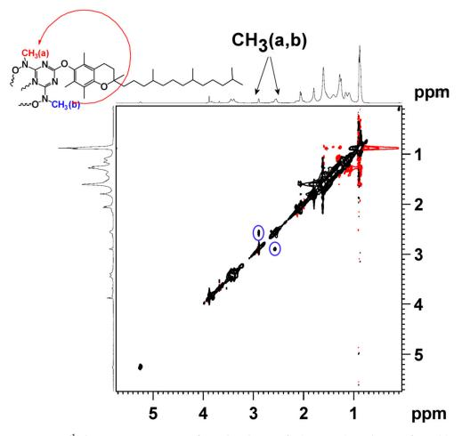
**Figure 3.** 2D {<sup>1</sup>H} grNOESY spectrum of CDCl<sub>3</sub> solution of **1** (1.00 mM). Exchange of CH<sub>3</sub>(a) and CH<sub>3</sub>(b) cross peaks in blue circles.
