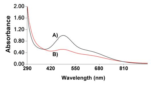
**Figure 8.** UV-vis spectra of DMSO- $d_6$ :D<sub>2</sub>O (1:9) solutions of 0.500 mM of (**A**) **1** [ $\lambda(\epsilon) = 490$  nm (2000 M<sup>-1</sup>cm<sup>-1</sup>), 675 nm (900 M<sup>-1</sup>cm<sup>-1</sup>)] and (**B**) **2** [ $\lambda(\epsilon) = 490$  nm (1100 M<sup>-1</sup>cm<sup>-1</sup>), 675 nm (660 M<sup>-1</sup>cm<sup>-1</sup>)].
