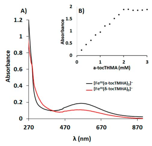
**Figure 5.** (A) UV-vis spectra of CHCl<sub>3</sub> solutions of 0.100 mM of **3** [black line,  $\lambda(\varepsilon) = 560$  nm (3200 M<sup>-1</sup> cm<sup>-1</sup>)] and **4** [red line,  $\lambda(\varepsilon) = 535$  nm (2200 M<sup>-1</sup> cm<sup>-1</sup>)]. (B) Absorbance at 560 nm vs. the concentration of *a*-tocTMHA added in the CHCl<sub>3</sub> solution of FeCl<sub>3</sub> (1.00 mM).
