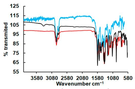
**Figure 1.** IR spectra of: **1** [*v*(V=O, 966 cm<sup>-1</sup>; (C=N triazine), 1579, 1529 cm<sup>-1</sup>; (Ph-O), 1242 cm<sup>-1</sup>; (N-O), 1092 cm<sup>-1</sup>]; 798 (V-O-V)] (black line), **2** [*v*(V=O, 966 cm<sup>-1</sup>; (C=N triazine), 1579, 1529 cm<sup>-1</sup>; (Ph-O), 1240 cm<sup>-1</sup>; (N-O), 1084 cm<sup>-1</sup>]; 798 (V-O-V) (red line), **3** [(C=N triazine), 1569, 1525 cm<sup>-1</sup>; (Ph-O), 1244 cm<sup>-1</sup>; (N-O), 1093 cm<sup>-1</sup>] (blue line).
