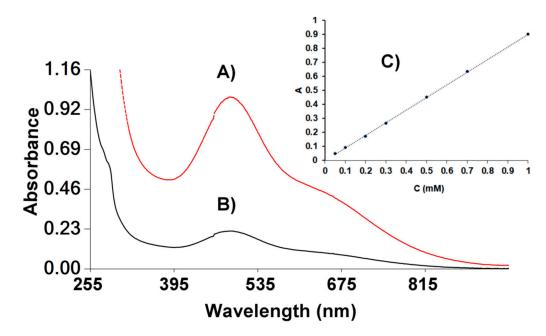
**Figure 9.** UV-vis spectra of DMSO- $d_6$ :D<sub>2</sub>O (1:9) solutions of **1** (**A**) 0.500 mM and (**B**) 0.100 mM, (**C**) graph of the absorption at 490 nm vs. concentration.
