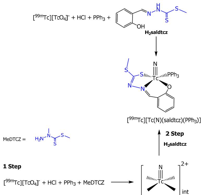
**Figure 10.** Reaction scheme for the synthesis of the  $[^{99m}\text{Tc}][\text{TcN}(\text{saldtcz})(\text{PPh}_3)]$  complex.
