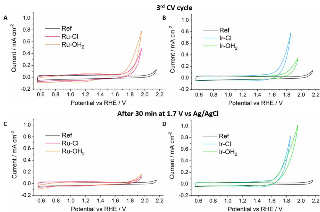
**Figure 3.** Top: Cyclic voltammetry (CV) scans of Ru-Cl (pink), Ru-OH<sub>2</sub> (orange) (A), Ir-Cl (blue) and Ir-OH<sub>2</sub> (green) (B) before chronoamperometry at 1.95 V vs. RHE. Bottom: CV scans of Ru-Cl (pink), Ru-OH<sub>2</sub> (orange) (C), Ir-Cl (blue) and Ir-OH<sub>2</sub> (green) (D) after chronoamperometry. CVs were recorded at 50 mV/s in 0.1 M  $\text{H}_2\text{SO}_4$  with a Pt counter electrode. Ref is meso-ITO with 30 cycles ALD-TiO<sub>2</sub>.
