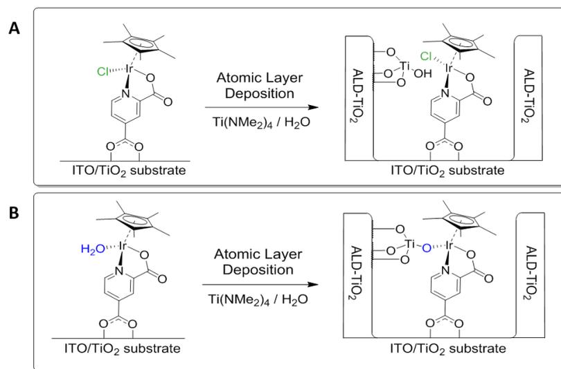
**Figure 4.** Reaction of anchored molecular Ir–Cl (A) and Ir–OH<sub>2</sub> (B) during the deposition of ALD-TiO<sub>2</sub> using TDMAT/water as precursors. Ir–Cl remains unchanged during ALD and is encapsulated in a TiO<sub>2</sub> layer, while Ir–OH<sub>2</sub> undergoes a reaction between the aqua ligand and the TDMAT, leading to a deactivated Ir complex embedded in TiO<sub>2</sub>.
