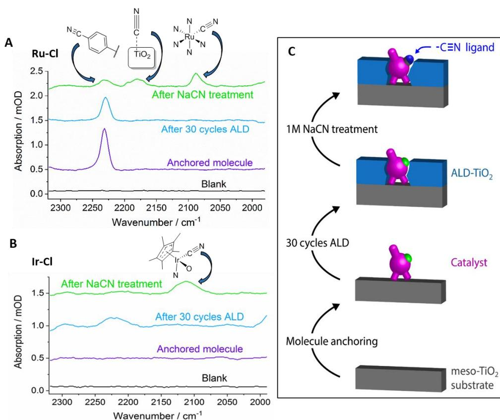
**Figure 2.** IR spectra of (A) Ru–Cl and (B) Ir–Cl adsorbed onto meso-TiO<sub>2</sub> after anchoring (purple), after ALD-TiO<sub>2</sub> deposition (blue) and after ligand exchange (green). (C) Schematic depiction of the process flow.
