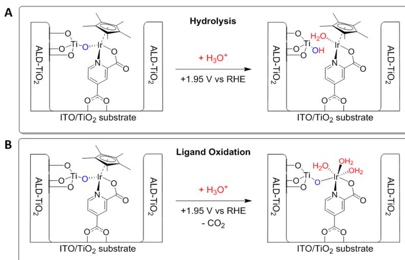
**Figure 5.** Proposed hydrolytic (A) and Cp\* ligand oxidation (B) mechanisms for (re)generation of the active Ir-OH<sub>2</sub> catalyst under operating conditions, which had undergone deactivation during the deposition of the ALD-TiO<sub>2</sub> layer.
