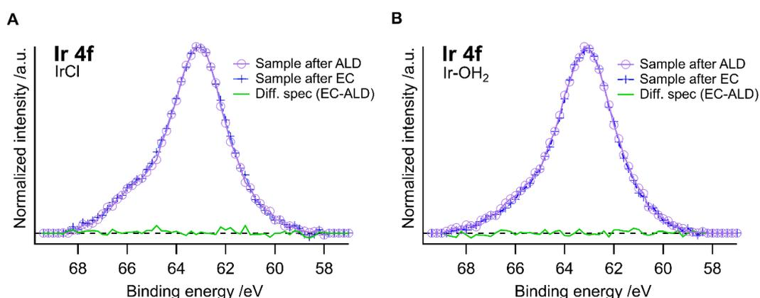
**Figure 6.** XPS spectra of (A) Ir-Cl and (B) Ir-OH<sub>2</sub> with ALD-TiO<sub>2</sub> before and after electrochemical measurements. The respective difference spectra are shown in green.
