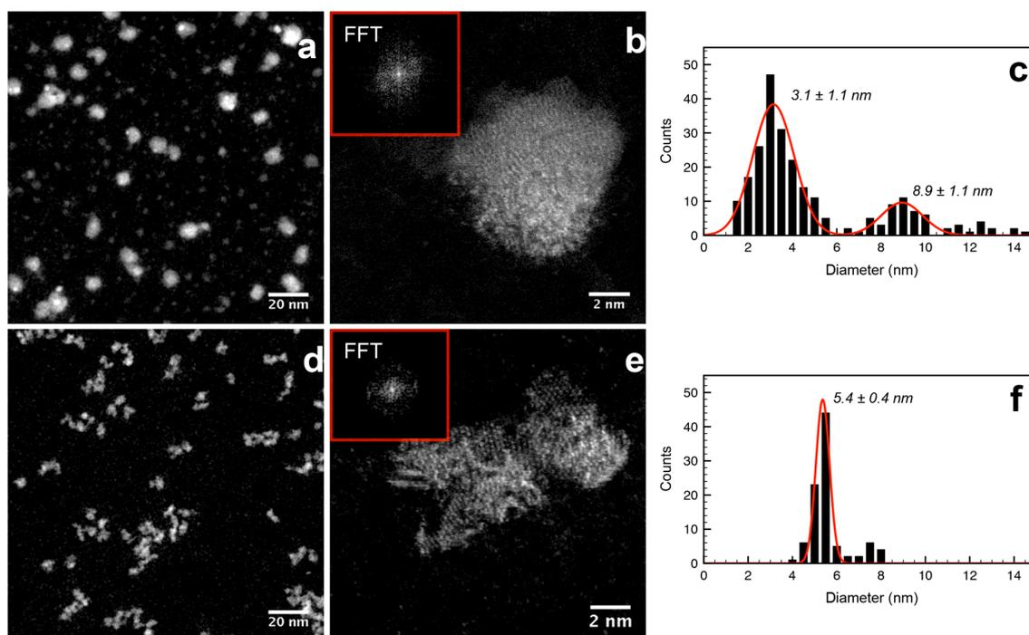
**Figure 3.** STEM images of MoS<sub>2</sub> clusters after (a,b) annealing only and (d,e) after sulphur addition only of as-deposited samples, (MoS<sub>2</sub>)<sub>1000</sub>; (c,f) are the corresponding size distributions of the clusters after annealing only and sulphur addition only, respectively.
