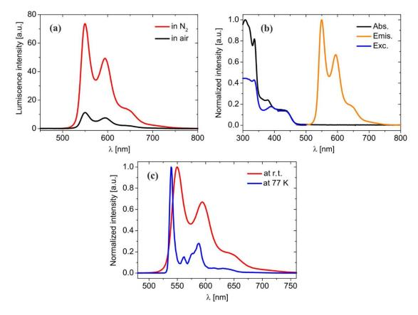
Figure 9. Emission spectra of aerated and deoxygenated solutions of 2 (a) in DCM recorded at  $\lambda_{\text{exc}} = 412$  nm; (b) comparison of the absorption, emission, and excitation spectra ( $\lambda = 550$  nm) of 2 in DCM at r. t.; (c) comparison of emission spectra of 2 at r. t. and at T = 77 K in a frozen 2-MeTHF matrix.
