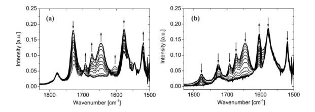
**Figure 8.** Spectroscopic changes in the IR during electrochemical reduction of complex 2 to  $2^{-}$  (a) and of  $2^{-}$  to  $2^{2^{-}}$  (b) in a 0.2 M NBu<sub>4</sub>PF<sub>6</sub>/THF solution at r. t.
