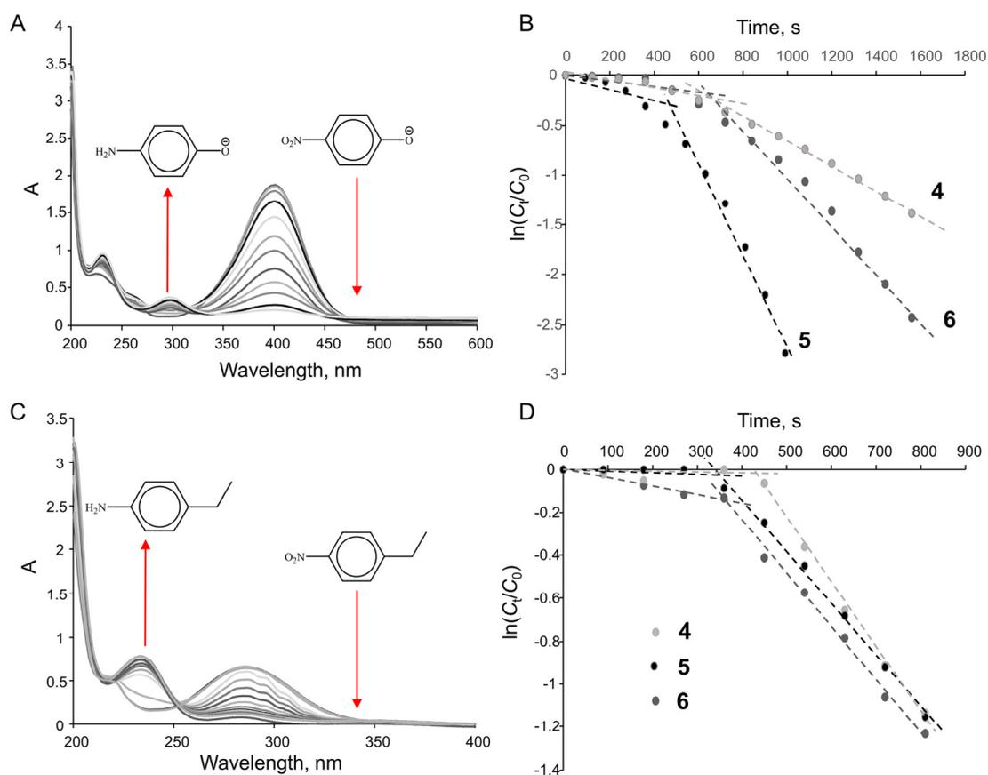
**Figure 3.** Changes in the UV-VIS spectrum during the reduction of (A) *p*-nitrophenol and (C) *p*-ethylnitrobenzene in the presence of 5; dependence of  $\ln(C_t/C_0)$  vs  $t$  in the presence of different complexes: (B) for *p*-nitrophenol and (D) *p*-ethylnitrobenzene. C (*p*-nitrophenol) = C (*p*-ethylnitrobenzene) = 0.1 mM, C (NaBH<sub>4</sub>) = 5 mM, C (4-6) = 0.002 mM, 0.1% THF-H<sub>2</sub>O, 21 °C, V = 2.5 mL, l = 10 mm.
