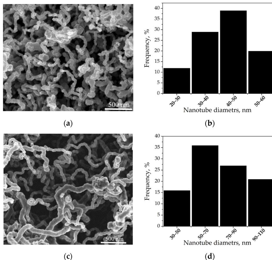
**Figure 2.** SEM images of the surface of the CNTAs and size distribution of grown nanotubes for CNTA 40 (a,b) and CNTA 75 (c,d).
