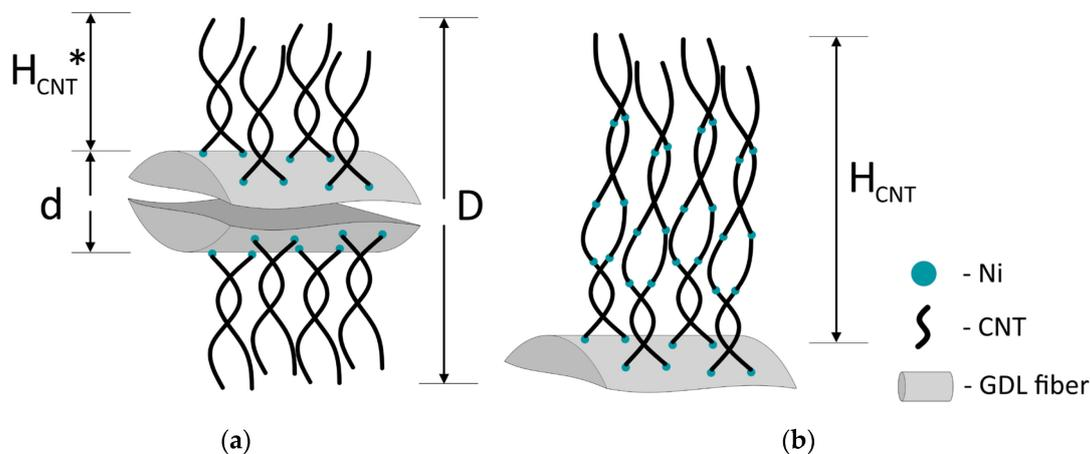
**Figure 7.** (a) Schematic representation of the CNTA growth on the GDL. CNTA on the fibers of the initial carbon GDL. (b) Layer-by-layer growth of the CNTA, where  $d$  is the diameter of the initial fiber,  $D$  is the diameter of the fiber with the CNTA (one-step growth),  $H_{CNT}^*$  is the one-layer (one-step growth) CNTA thickness, and  $H_{CNT}$  is the entire CNTA thickness. Symbols: blue dots are Ni particles, gray cylinder is the GDL fiber, and black line is CNT.
