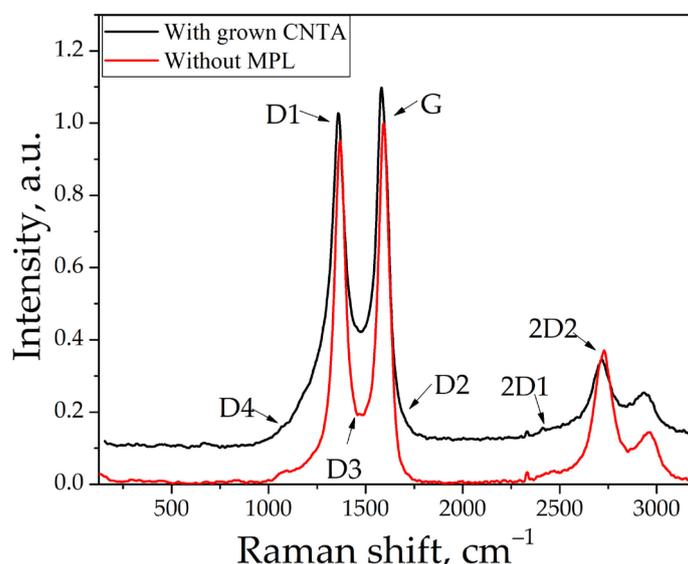
**Figure 4.** Raman spectra of ELAT LT 1400 cloth without MPL and with the grown CNTA 50.
