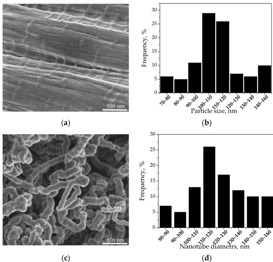
**Figure 1.** SEM image of the GDL with the Ni catalyst (a), size distribution of Ni agglomerates (b), SEM image of the grown CNTs (c), and size distribution of CNTs diameters for the CNTA 120 sample (d).
