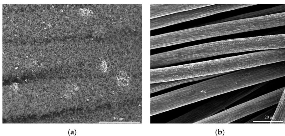
**Figure 3.** SEM images of GDL carbon fibers with (a) and without (b) CNTA 40. The thickness of the array is 4 μm.
