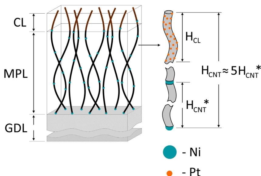
**Figure 8.** Schematic of the obtained CNTA-based electrode, where particles of the Ni catalyst used for the CNT growth are marked in blue, the platinum catalyst particles are marked in red,  $H_{CL}$  is the height of the catalytic layer,  $H_{CNT}$  is the height of the entire microporous layer of the CNTA, and  $H_{CNT}^*$  is the height of one layer obtained by a single CNT synthesis.
