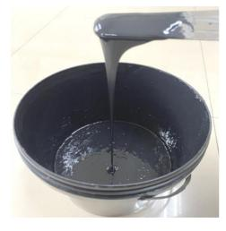
Figure 11. Photo of glass enamel paste to be printed on automobile glass.
