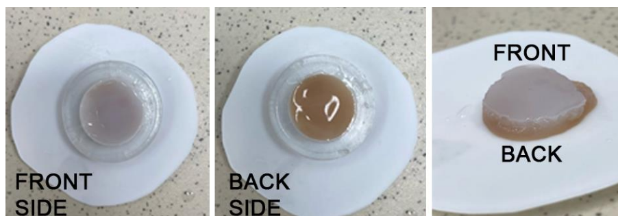
Figure S10. The images of the front (irradiated) and back (nonirradiated) sides of the PAAm@Mo 132 @TiO 2 hydrogel after the UV irradiation for 3 h in the aqueous solution.
