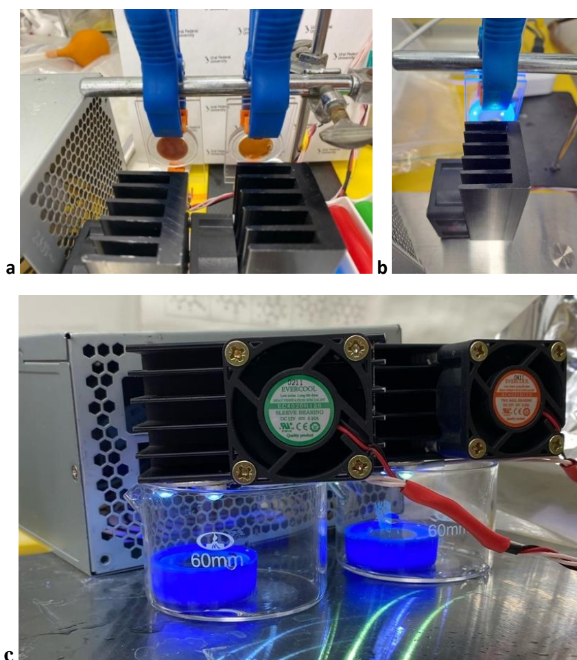
Figure S4. Experimental setups for hydrogel irradiation. Each UV-LED module (UV-module) has 3 LED emitting light at 365 nm with 3W per each LED giving 9W in sum. (a) and (b) – the setups for irradiation hydrogel in cell as prepared; (c) – the setup for hydrogel irradiation within PVC-ring in water media. The blue caps were used to prevent any reflection of UV light to avoid indirect irradiation of hydrogel's back side. The water volume and distance to UV-module was the same for both hydrogels (PAAm@Mo 132 and PAAm@Mo 132 @TiO 2 ).
