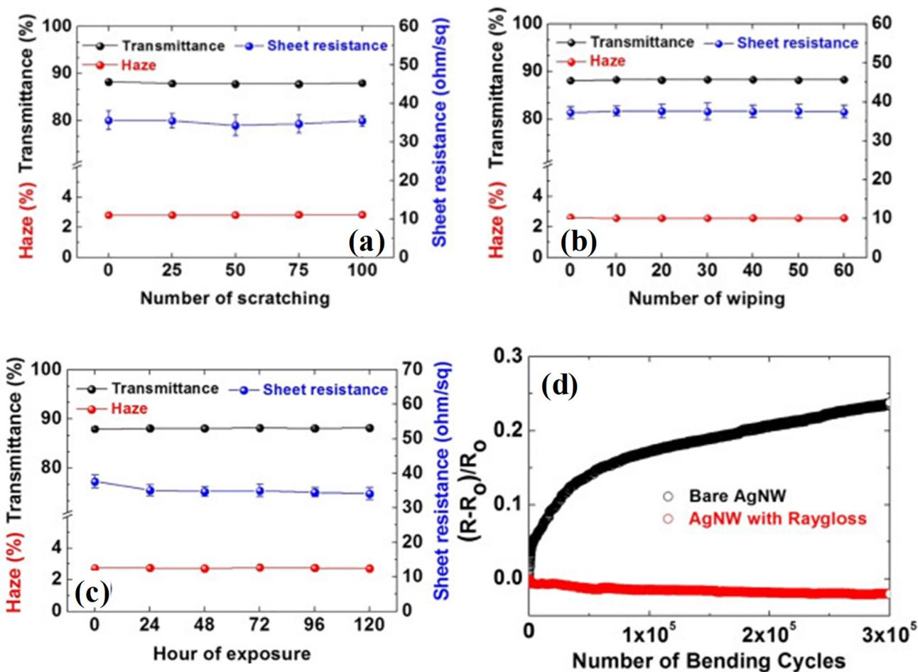
**Figure 2.** Change in optical transmittance, haze, and sheet resistance as a function of (a) the number of scratches made using a pen, (b) the number of wipes using IPA, (c) the hours of exposure to ambient air at 85 °C, and (d) the number of bending cycles of PU coating on the AgNW electrodes. Reproduced with permission from ref. [33].
