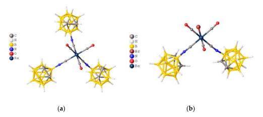
**Figure 35.** Structures of complexes (a)  $[Re(CO)_3(3-CN-1,2-B_{10}C_2H_{10})_3][PF_6]$  (anion is omitted) and (b)  $[Re(CO)_3(3-CN-1,2-B_{10}C_2H_{10})_2Br]$ .
