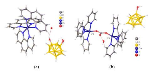
Figure 5. Structures of (a)  $[Ni(Phen)_3][B_{10}H_9OH]\cdot 0.75CH_3CN\cdot 0.5H_2O$  and (b)  $[Cu_2(bipy)_4(\mu-CO_3)][2-B_{10}H_9OH]\cdot 2DMSO\cdot H_2O$ .
