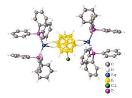
Figure 3. Structure of binuclear silver(I) complex [Ag<sub>2</sub>(Ph<sub>3</sub>P)<sub>4</sub>[B<sub>12</sub>H<sub>11</sub>Cl]].
