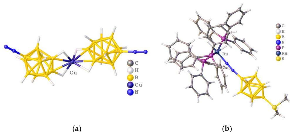
**Figure 14.** (a) Anionic copper(I) complex in  $[\text{Et}_3\text{NH}][\text{Cu}[1\text{-B}_{10}\text{H}_9\text{N}_2]_2]$  and (b) molecular ruthenium(II) complex  $[\text{RuH}_2[\text{N}_2\text{B}_{10}\text{H}_8\text{SMe}_2](\text{Ph}_3\text{P})_3] \cdot 3\text{C}_6\text{H}_6$ .
