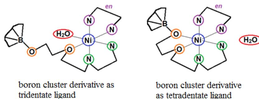
**Figure 11.** Schematic representations of the structures of nickel(II) complexes  $[\text{Ni}(\text{H}_2\text{O})(\text{en})_3[2\text{-B}_{10}\text{H}_9\text{O}(\text{CH}_2)_2\text{O}(\text{CH}_2)_2\text{NH}(\text{CH}_2)_2\text{NH}_2]]$  (left) and  $[\text{Ni}(\text{en})[2\text{-B}_{10}\text{H}_9\text{O}(\text{CH}_2)_2\text{O}(\text{CH}_2)_2\text{NH}(\text{CH}_2)_2\text{NH}_2]] \cdot \text{H}_2\text{O}$  (right).
