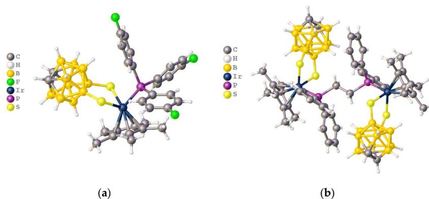
**Figure 32.** Structures of iridium complexes (a)  $[\text{Cp}^*\text{Ir}((4\text{-F-C}_6\text{H}_4)_3\text{P})\{9,10\text{-S}_2\text{C}_2\text{B}_{10}\text{H}_{10}\}]$  and (b)  $[\text{Cp}^*\text{Ir}(\text{Ph}_2\text{PCH}_2)\{9,10\text{-S}_2\text{C}_2\text{B}_{10}\text{H}_{10}\}]_2$ .
