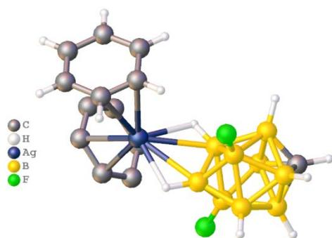
Figure 23. Structure of silver(I) complex  $[\text{Ag}(\text{C}_6\text{H}_6)_2][6,8\text{-CB}_9\text{H}_8\text{F}_2]$ .
