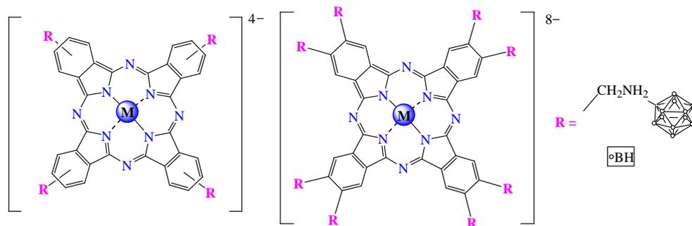
**Figure 19.** Structures of cobalt(II) and aluminum(III) complexes with the *closo*-dodecaborate derivatives of phthalocyanine containing B–N bonds (M = Co or Al(OH)).
