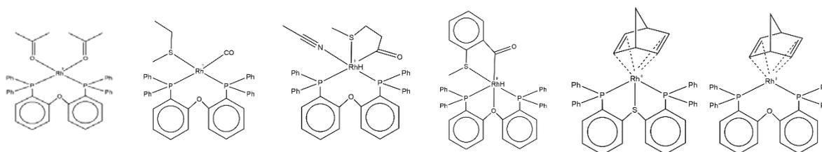
**Scheme 6.** Structures of ligands in complexes  $[\text{RhL}][\text{CB}_{11}\text{H}_6\text{Hal}_6]$  (Hal = Cl, Br).
