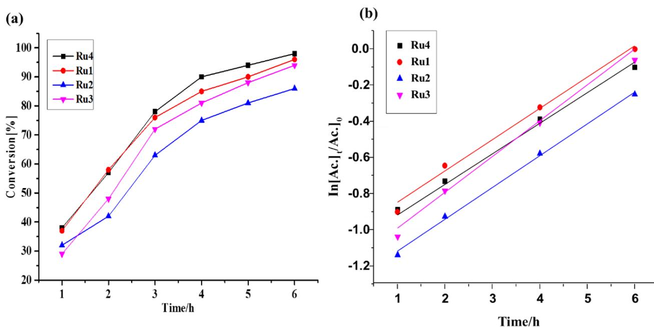
**Figure 3.** Time-dependent transfer hydrogenation reaction of acetophenone catalysed by **Ru1–Ru4**,  $5.00 \times 10^{-3}$  mol% (50 ppm);  $t\text{BuOK}$ : 4.0 mol%; temp. 82 °C). (a) Yield (%) vs. time graph, (b)  $-\ln[\text{Ac.}]_t/[\text{Ac.}]_0$  vs. time plot of the **Ru1–Ru4** catalysts (Ac.—acetophenone).
