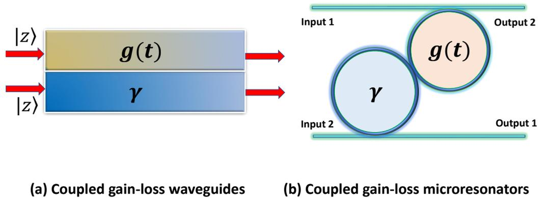
**Figure 1.** Exemplary setups, as the coupled waveguides and the coupled microresonators driven by a coherent field, which carry gain–loss media. The inputs  $|z\rangle$  are squeezed vacuum or squeeze coherent states. The gain, loss, and coupling are denoted by  $g$ ,  $\gamma$ , and  $J$ , respectively.
