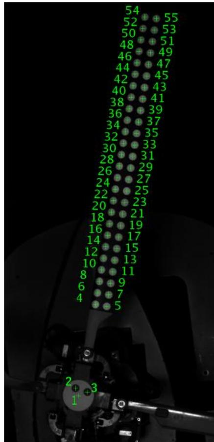
**Figure 9.** Numbering of all targets on the rotor.
