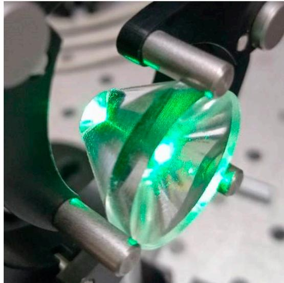
**Figure 7.** Appearance of the fabricated bi-conic axicon.
