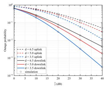
**Figure 5.** Outage probability under different FSO communication distance when  $\gamma_{th} = 0$  dB,  $\xi = 10$ , N = 10.
