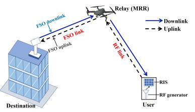
Figure 1. A mixed RF/FSO UAV communication system based on MRR and RIS.
