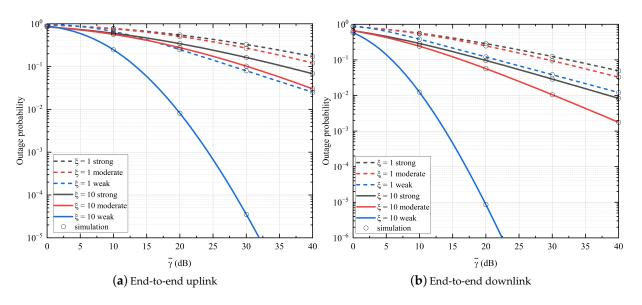
**Figure 4.** Outage probability under different atmospheric turbulence and pointing error when  $\gamma_{th} = 0 \text{ dB}, \xi = 10, N = 10, d = 5.0 \text{ km}.$
