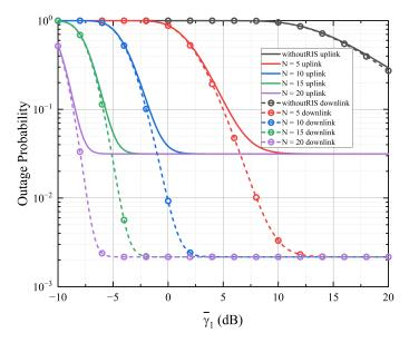
**Figure 3.** Outage probability with different *N* when  $\gamma_{th} = 15 \text{ dB}$ ,  $\alpha = 4.0$ ,  $\beta = 1.6$ ,  $\xi = 10$ ,  $\overline{\gamma}_2 = 50 \text{ dB}$ , d = 5.0 km.
