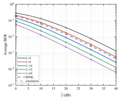
**Figure 6.** Average BER of end-to-end downlink under different *L* when  $\alpha = 4.0$ ,  $\beta = 1.6$ ,  $\xi = 10$ , d = 5.0 km, N = 10.
