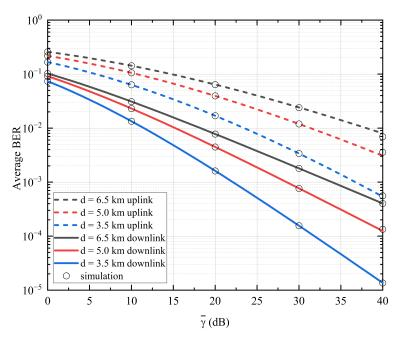
**Figure 9.** Average BER under different FSO communication distance when  $\xi = 10$ , L = 32, N = 10.
