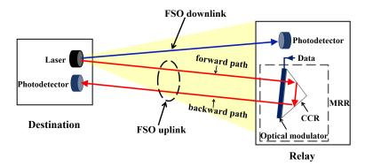
Figure 2. Schematic diagram of MRR FSO with bidirectional communication.
