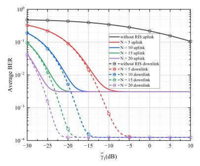
**Figure 7.** Average BER with different *N* when  $\alpha = 4.0$ ,  $\beta = 1.6$ ,  $\xi = 10$ ,  $\overline{\gamma}_2 = 40$  dB, d = 5.0 km, L = 32.
