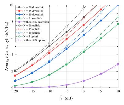
**Figure 10.** Average channel capacity under different *N* when  $\alpha = 4.0$ ,  $\beta = 1.6$ ,  $\xi = 10$ ,  $\overline{\gamma}_2 = 40$  dB, d = 5.0 km.
