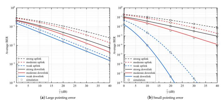
**Figure 8.** Average BER under different pointing error and atmospheric turbulence when d = 5.0 km, L = 32, N = 10.
