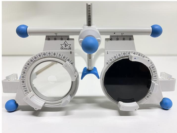
**Figure 1.** Trial frame example with the 0.4 Bangerter foil pasted on a plane lens, while the clear central aperture is centered to the lens, inserted at the back side of the trial frame—in front of the right eye. The slots on the front side were reserved for the individual sphero-cylindrical correction and the near compensation lens. The infrared filter on the left eye was used to measure the pupil size.
