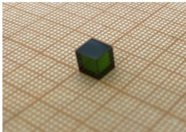
**Figure 1.** Image of the studied crystal  $\text{LiTaO}_3:\text{Cr}(0.2):\text{Nd}(0.45 \text{ wt}\%)$ .
