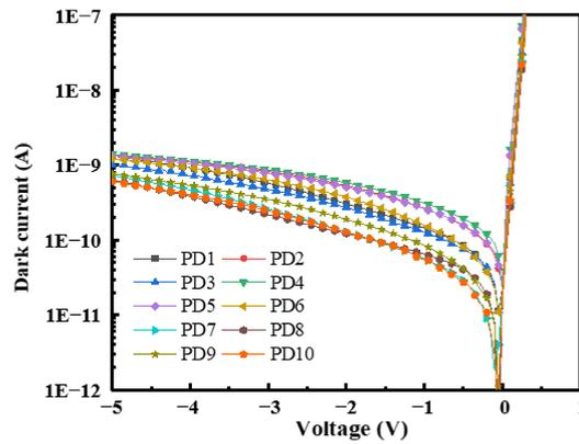
Figure 4. The dark current measurement result of the photodetector array.
