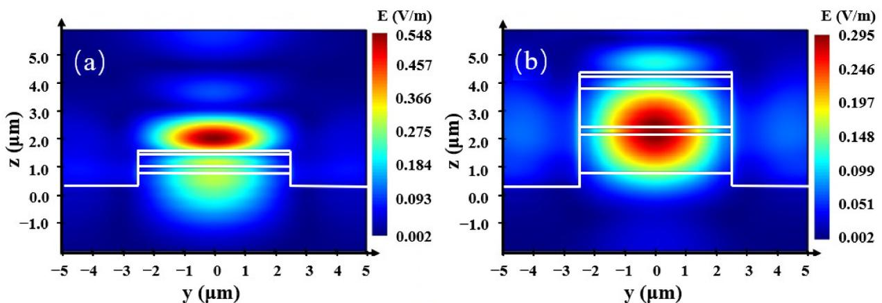
**Figure 2.** Cross-section of the waveguide photodetector (WGPD) with different  $\text{InGa}_{0.24}\text{As}_{0.53}\text{P}$  layer thicknesses: (a) 0  $\mu\text{m}$  thick  $\text{InGa}_{0.24}\text{As}_{0.53}\text{P}$  layer and 0.2  $\mu\text{m}$  thick  $\text{In}_{0.53}\text{Ga}_{0.47}\text{As}$  layer. (b) 1.4  $\mu\text{m}$  thick  $\text{InGa}_{0.24}\text{As}_{0.53}\text{P}$  layer and 0.2  $\mu\text{m}$  thick  $\text{In}_{0.53}\text{Ga}_{0.47}\text{As}$  layer.
