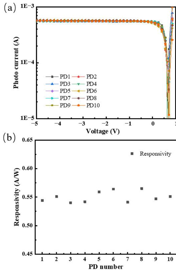
Figure 5. (a) The photocurrent measurement result of the photodetector array as a function of voltage bias without an anti-reflection (AR) coating, (b) The responsivity result of the photodetector array without an anti-reflection (AR) coating.
