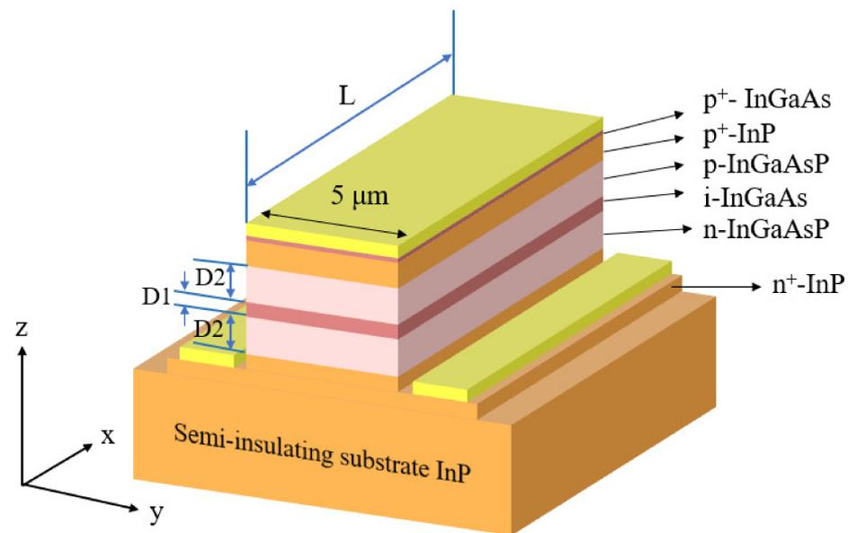
Figure 1. The three-dimensional schematic structure of the single photodetector (PD).
