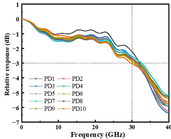
Figure 6. Frequency response measurement result of the photodetector (PD) array at 5 V reverse bias.
