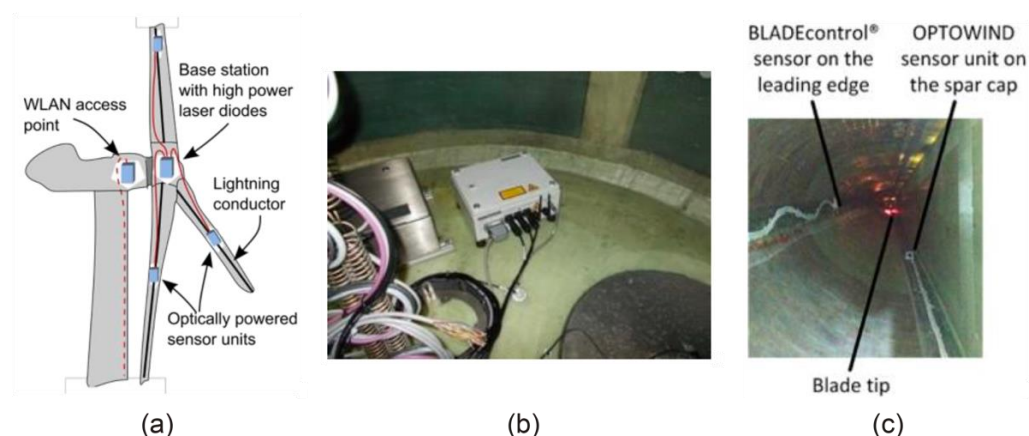
Figure 4. (a) Configuration of optically powered rotor blade condition monitoring system. Photographs of (b) base station placed inside of hub of wind turbine and (c) inside of rotor blade [33].
