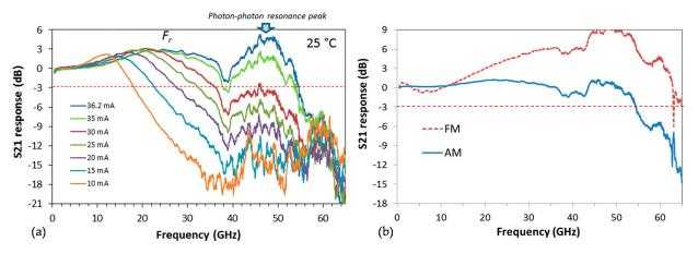
**Figure 2.** (a) S<sub>21</sub> amplitude responses for a bias range from 10–36.2 mA at 25°C; (b) S<sub>21</sub> amplitude and frequency responses at 36.2 mA gain bias at 25°C; FM: Frequency modulation; AM: Amplitude modulation; (From [46], © 2017 IEEE).
