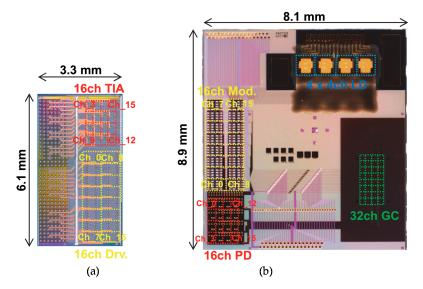
**Figure 11.** Photographs of (**a**) electronic integrated circuit (EIC) and (**b**) photonic integrated circuit (PIC) of the high-density 16 channels optical transceivers where transmitter and receiver elements were highly integrated in the chips;  $4 \times 4$  channels laser diodes (LDs) were assembled and 32 channels (32ch) grating couplers (GCs) were formed in the PIC; Ch\_1: the first channel; Ch\_2: the second channel; TIA: trans-impedance amplifier; (From [28] © 2021 IEEE).
