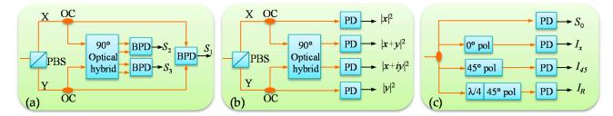
**Figure 6.** Different structures of Stokes vector direct detection: (**a**) structure I [19]; (**b**) structure II; (**c**) structure III [21]; PBS: polarization beam splitter; OC: optical coupler; BPD: balanced photodetector; pol: polarizer.
