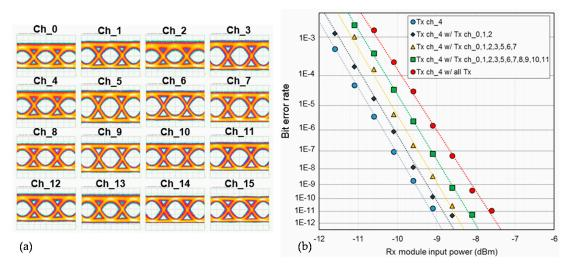
**Figure 12.** (a) Optical eye diagrams of all transmitter channels and (b) the sensitivity changes of ch\_4 at multi-channel transmitters operations; Ch\_1: the first channel; TX: transmitter; Rx: receiver; (From [28] © 2021 IEEE).
