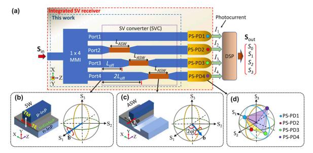
**Figure 7.** (a) Schematic top-view (XZ-plane) of the integrated Stokes vector receiver on InP; (b) symmetric waveguide (SW) and (c) asymmetric waveguide (ASW) used in the receiver; (d) illustrations of four basis vectors on the Poincaré sphere; MMI: multimode interference; SV: Stokes vector; PS-PD: polarization-selective PD; TE: transverse-electric; TM: transverse-magnetic; (From [106] © 2021 OSA).
