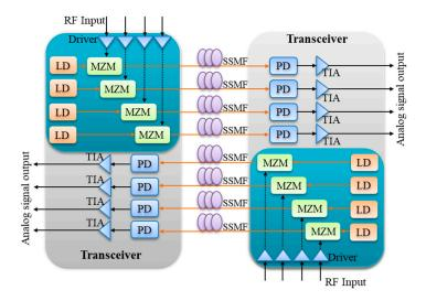
**Figure 10.** Block diagram of transceiver integration scheme based on direct detection. LD: laser diode; MZM: Mach-Zehnder modulator; RF: radio-frequency; SSMF: standard single mode fiber; TIA: trans-impedance amplifier; PD: photodetector.
