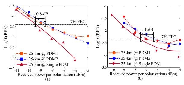
**Figure 9.** Twenty-five km transmission performance of the 2 × PDM-PAM4 and the single PDM-PAM4 systems. (a) BER at 4 × 20-Gbit/s and (b) 4 × 40-Gbit/s. PDM: polarization division multiplexing; FEC: forward error correction; (From [101]  $\bigcirc$  2021 OSA).
