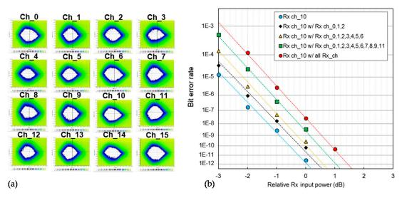
**Figure 13.** (a) Optical eye diagrams of all receiver channels and (b) BER performance under the first channel; TX: transmitter; Rx: receiver; (From [28] © 2021 IEEE).
