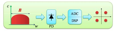
**Figure 5.** Kramers-Kronig direct detection scheme; PD: photodetector; ADC: analog to digital converter; DSP: digital signal processing module.
