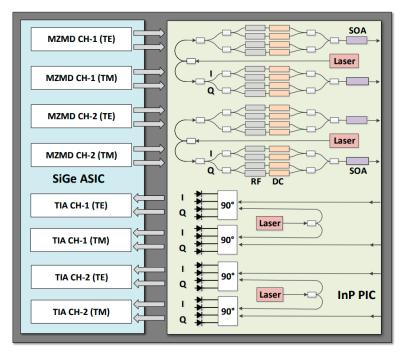
**Figure 14.** Schematic of transceiver integration scheme based on coherent detection; MZMD: Mach Zehnder modulator driver; TE: transverse-electric; TM: transverse-magnetic; TIA: transimpedance amplifier; RF: radio-frequency; DC: direct current; InP: Indium phosphide; PIC: photonic integrated circuit; SOA: semiconductor optical amplifier; Ch\_1: the first channel; (From [27] © 2021 IEEE).
