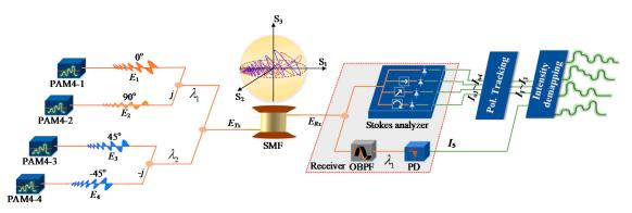
**Figure 8.** The principle of the simplified detection scheme. PAM: pulse amplitude modulation; SMF: single mode fiber; Pol.: polarization; OBPF: optical band-pass filter; PD, photodetector; (From [103] © 2021 OSA).
