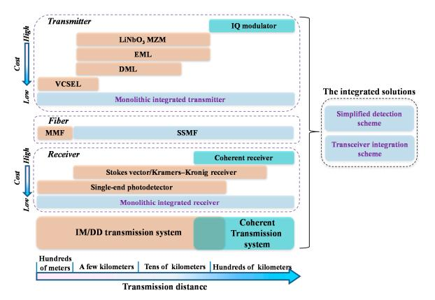
Figure 16. The technological and component options for high-speed short-reach transmission systems.
