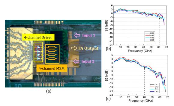
**Figure 4.** (a) Micrograph of the chip-on-board silicon photonics transmitter; (b)  $S_{21}$  characteristics of silicon photonics modulator under different channels (e.g., CH\_1, CH\_2, CH\_3, and CH\_4); (c)  $S_{21}$  characteristics of transmitter co-packaged with the driver under different channels. FA: fiber array; (From [88] © 2021 Chinese Laser Press).
