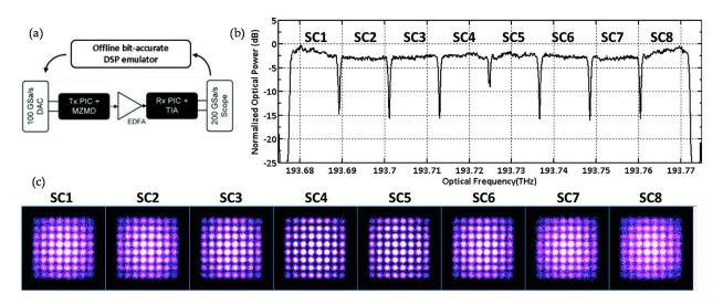
**Figure 15.** (a) Experimental setup for 800-Gbit/s transmission measurements; (b) optical spectra showing a single ~95-GHz wide channel with eight digital subcarriers (from SC1 to SC8); (c) all received eight subcarrier probabilistic shaping 64-QAM constellations; DAC: digital to analog converter; Table 1. the first subcarrier; DSP: digital signal processing; MZMD: Mach Zehnder modulator driver; PIC: photonic integrated circuit; TIA: trans-impedance amplifier; (From [27] © 2021 IEEE).
