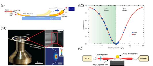
gion (Figure 3c) [65]. A 1.6- $\mu$ m-diameter As<sub>2</sub>S<sub>3</sub> fiber taper was used for near-field coupling with ChG microspheres with the coupling loss less than 3 dB over 4.465–4.705  $\mu$ m.
