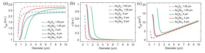
**Figure 2.** Numerical solutions of diameter-dependent (**a**) effective refractive index ( $n_{eff}$ ), (**b**) fractional evanescent fields ( $\eta$ ), and (**c**) effective mode area ( $A_{eff}$ ) of As<sub>2</sub>S<sub>3</sub> and As<sub>2</sub>Se<sub>3</sub> MFs at wavelengths of 1.55 µm, 4 µm, and 8 µm, respectively.
