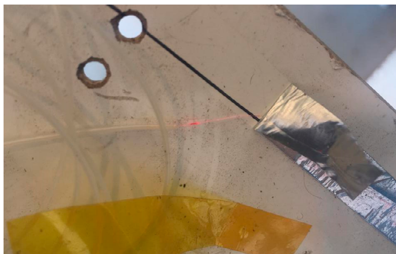
Figure 21. Light escaping the fibre at a microcrack; visibility produced by the VFL.
