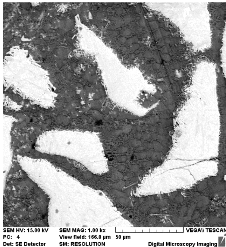
Figure 5. A view of crack propagation in carbide particle of LD-thick layer.
