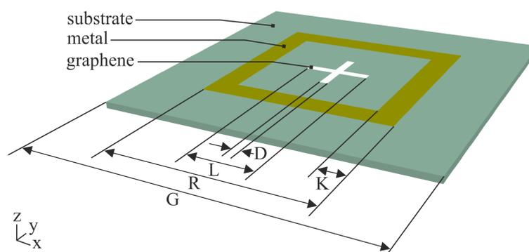
**Figure 1.** Scheme of the unit cell geometry: The graphene cross-like layer is located on the quartz substrate (with  $\epsilon = 3.75$ ) in its center and is surrounded by a square gold ring.  $G$  is the size of the unit cell,  $R$  and  $K$  is the external size and width of gold ring respectively, and  $L$  and  $D$  is the length and the width of graphene cross-like layer respectively.
