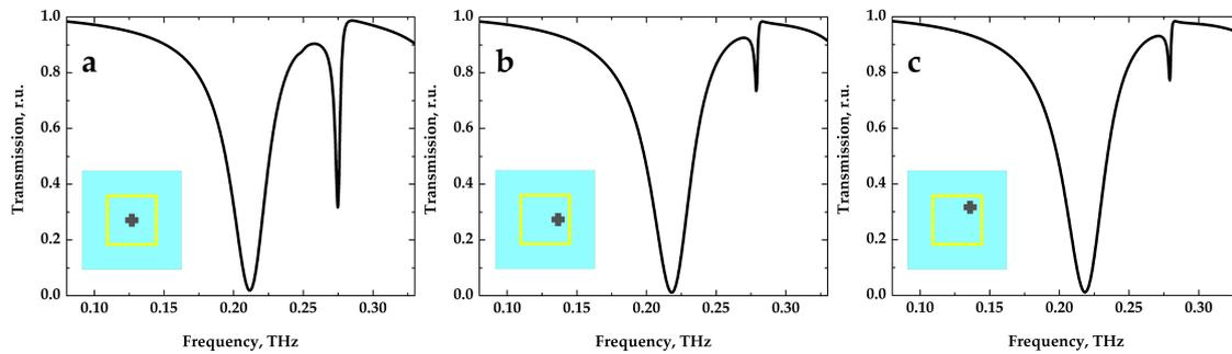
**Figure 5.** Transmission spectra of the filter with different unit cell structure: Original designed filter structure (a), structure with shifted graphene cross along one direction up to 100  $\mu\text{m}$  (b), structure with shifted graphene cross along two directions up to 100  $\mu\text{m}$ , and (c) graphene Fermi energy fixed at 0.5 eV.
