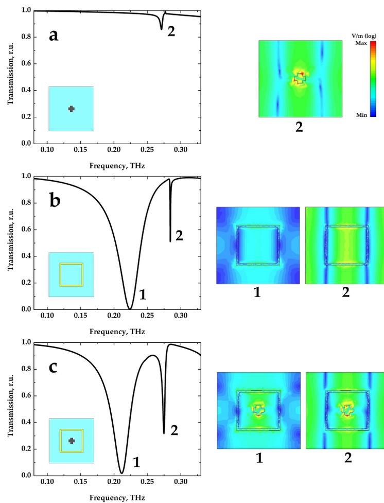
**Figure 2.** On the left side: Transmittance spectra of the filter in the absence of the gold ring with a fixed graphene Fermi level of 0.5 eV (a), in the absence of the graphene layer (b), and in case of the full Fano-resonant structure under electrostatic doping of 0.5 eV (c). On the right side: Corresponding electric field distributions.
