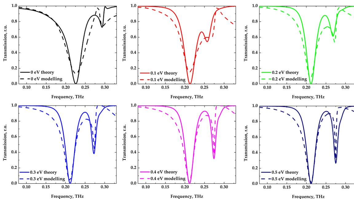
**Figure 4.** Transmission spectra for theoretical and numerical calculations with increasing graphene Fermi level values from 0 eV to 0.5 eV (different gate voltage values) for graphene-based filter.
