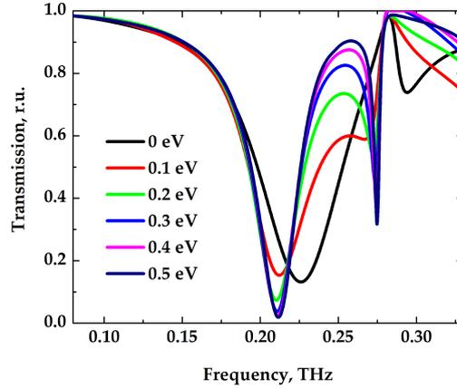
**Figure 3.** Transmission spectra of the filter for the different graphene Fermi level values from 0 eV to 0.5 eV (different gate voltage values).
