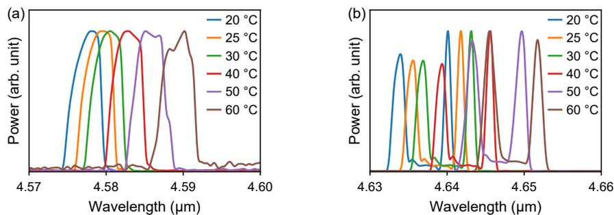
**Figure 7.** Normalized spectral dependence on the temperature for (a) a DFB laser from channel 2 with a 200 ns drive pulse width and (b) a DBR laser from channel 5 with a 100 ns drive pulse width. Heating during the pulse limits the linewidth of each mode.
