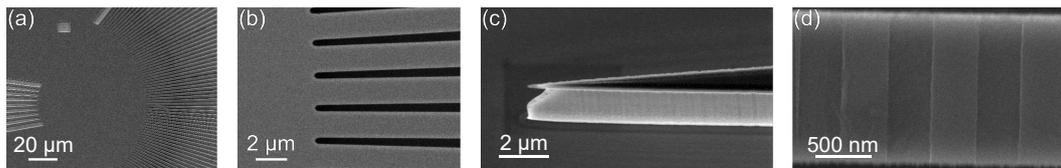
**Figure 3.** SEMs of the (a) star coupler of an AWG, (b) transition between the free-propagation region of the star coupler to the arrayed waveguides of an AWG, (c) slanted view of a QCL taper tip before etching the  $n$ -QC structure, where the top layer is the  $\text{SiO}_2$  hardmask, and (d) a grating etched in the top of a Si waveguide before bonding the QCL.
