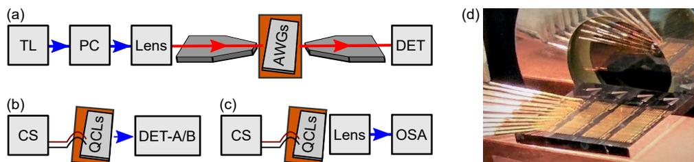
**Figure 4.** Experimental setups for (a) the AWG passive transmission, (b) the QCL LIV characteristics, and (c) the QCL spectral measurements. CS represents a current source and PC represents a polarization controller. (d) A photograph of the QCL array coupled to an AWG with the output collected by DET-A, corresponding to the schematic in (b).
