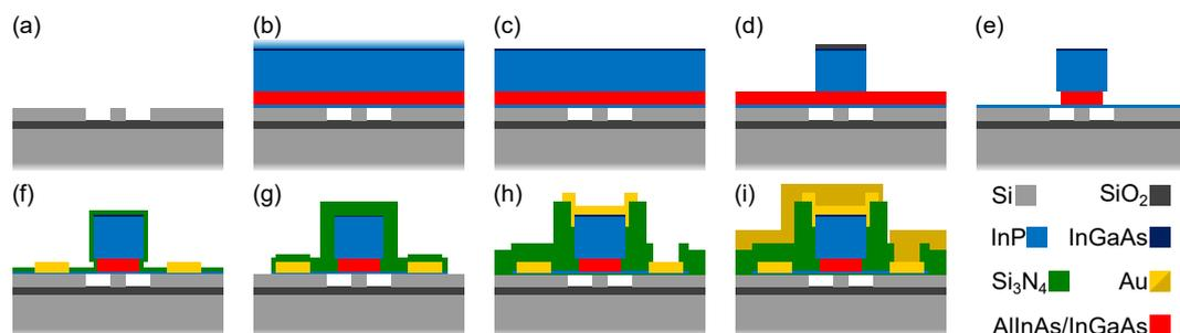
**Figure 2.** Processing steps: (a) gratings and Si waveguides are defined; (b) the QCL chip is bonded to the Si wafer; (c) the InP substrate is removed; (d) top contact and cladding layers are dry etched; (e) the active region is wet etched; (f) the bottom contact region is defined and gold is deposited; (g)  $\text{Si}_3\text{N}_4$  is deposited and the bottom contact layer is etched; (h) vias are etched and the top contact metal is deposited; (i) probe metal is deposited.
