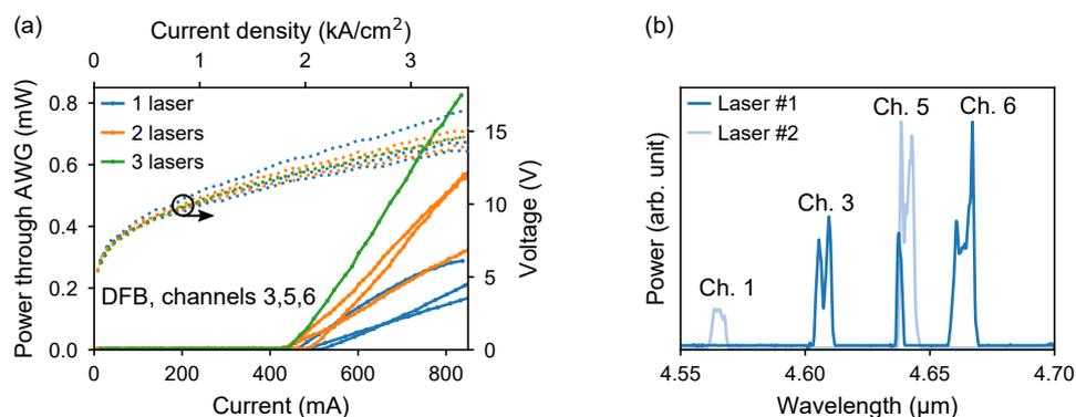
**Figure 10.** (a) LIV plots of a multi-spectral three-channel DFB while driving laser channels 3, 5, and 6. (b) Spectra of the three-channel DFB laser (Laser #1) and another two-channel DFB laser (Laser #2).
