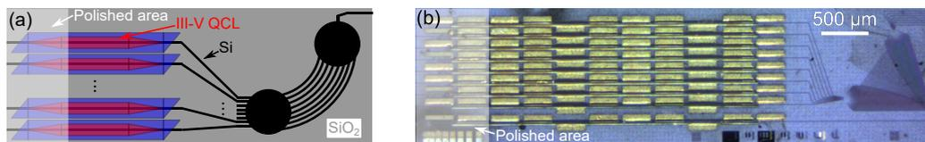
**Figure 1.** (a) Top-view schematic of the QCL array and arrayed waveguide grating (AWG). Mirrors are defined under the red III-V QCL ridges for both the distributed feedback (DFB) and distributed Bragg-reflection (DBR) type lasers. (b) Micrograph of a multi-spectral DFB laser, showing the individual lasers on the left and the AWG combiner on the right.
