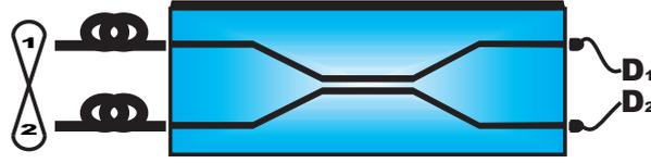
**Figure 8.** Integrated detection system. The device is made up of a 3 dB DC and two PNRDs. The difference of the number of photons recorded at each output  $D_1$  and  $D_2$  gives information about the order and handedness of the input quantum vortex state.
