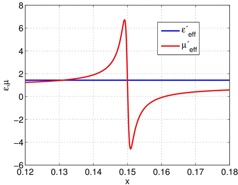
**Figure 2.** Effective parameters  $\mu'_{\text{eff}}$  and  $\epsilon'_{\text{eff}}$  of a lattice of all-dielectric RA cylinders with  $\epsilon_{\rho} = 1$ ,  $\epsilon_{\varphi} = 253$  and  $\mu_z = 1$  with area fraction  $p = 0.2$ . The lattice exhibits artificial magnetism, and even negative values of  $\mu'_{\text{eff}}$  are achieved.
