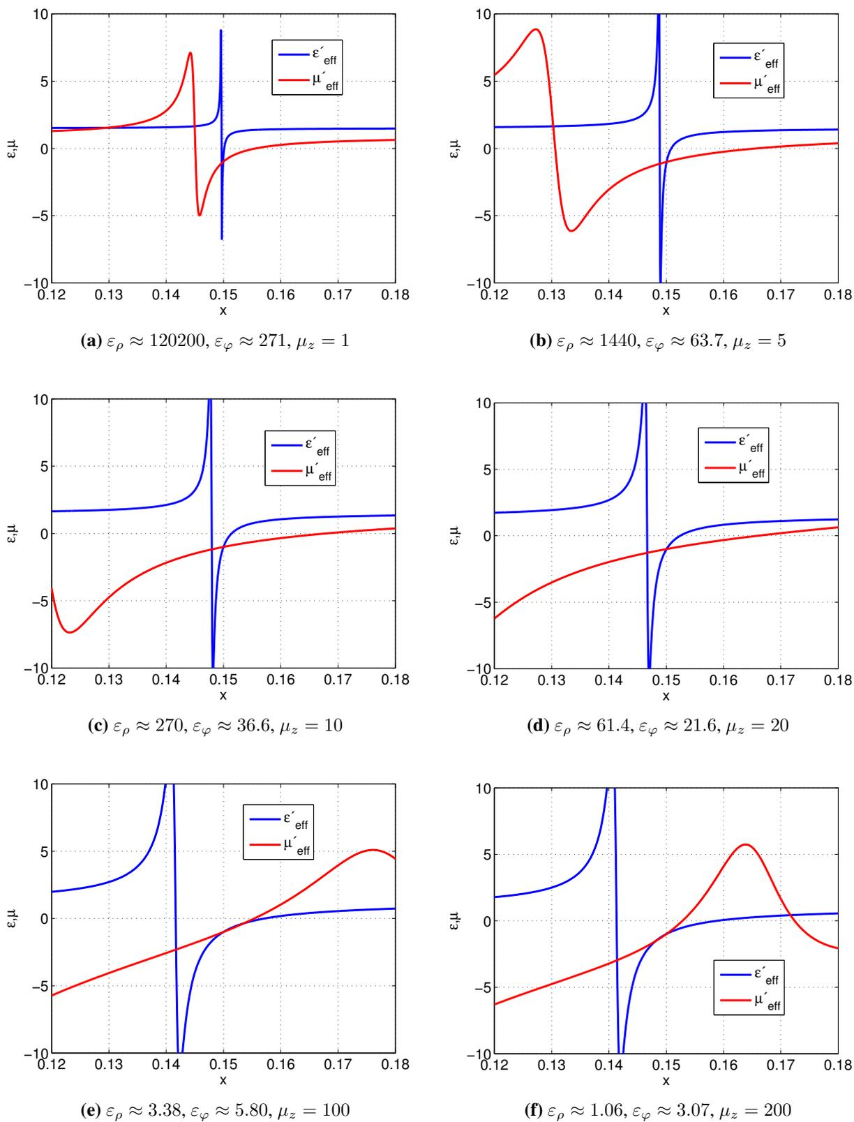
**Figure 3.** Effective parameters  $\mu'_{\text{eff}}$  and  $\epsilon'_{\text{eff}}$  of a lattice of magnetodielectric RA cylinders with area fraction  $p = 0.2$ . All configurations 3a–3f yield  $\epsilon'_{\text{eff}} = \mu'_{\text{eff}} = -1$  at  $x = 0.15$ .
