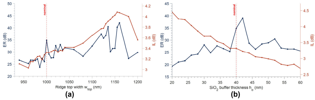
Figure 7. Fabrication tolerance of the polarizer to the two dielectric geometric parameters at the optimized point ( \theta = 78^\circ , h_m = 13 nm, \lambda = 1550 nm, T = 25^\circ\text{C} ); PER (left axis, blue) and IL (right axis, orange). (a) Ridge top width w_{top} over 940–1200 nm; (b) SiO 2 buffer thickness h_o over 20–60 nm. The dotted line marks the nominal value.
