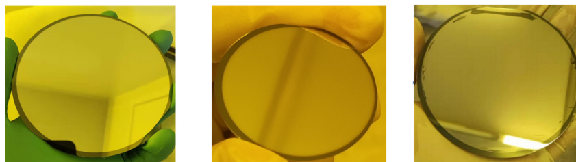
Figure 4. Representative peeling results of neat PVA films deposited on ultrathin Ag films under different intrinsic material parameters, including degree of polymerization, degree of hydrolysis, and solution solid content. Variations in these parameters lead to either excessive interfacial adhesion with partial Ag film damage or insufficient bulk cohesion accompanied by cohesive failure and polymer residues, indicating a trade-off between interfacial adhesion and bulk cohesion in neat PVA systems. The circled regions highlight areas of partial Ag film damage.
