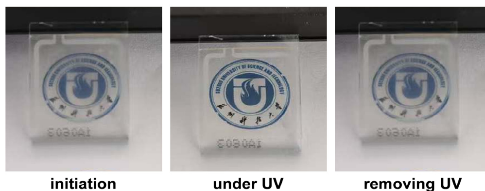
Figure 11. Visual demonstration of the photo-switching capability. The background of the liquid crystal cells is the emblem of the authors' university, and the non-English characters indicate the Chinese name of the university.
