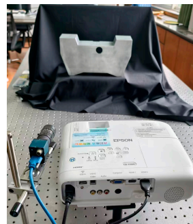
Figure 7. Experimental setup of the FPP system, including a digital projector, a CMOS camera, a stepped calibration target, and an optical breadboard.
