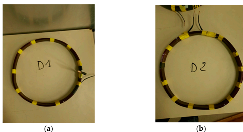
Figure 3. Defective winding 1 (D1) in (a) and defective winding 2 (D2) in (b).
