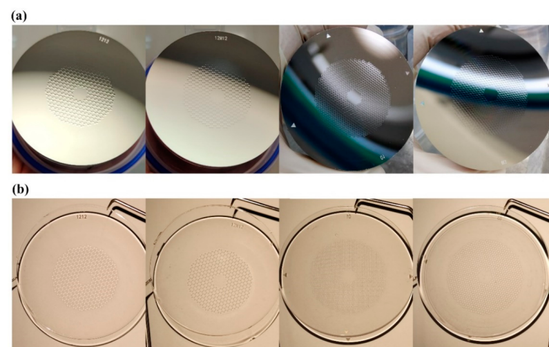
Figure 9. Injection molding of both LARI and HOPE spectacle lenses with aperture size of 75 mm in diameter. From left to right: PLARI, NLARI, O-HOPE, and T-HOPE. (a) Mold inserts manufactured by high-precision single-point diamond turning; (b) molded spectacle lenses under illumination.
