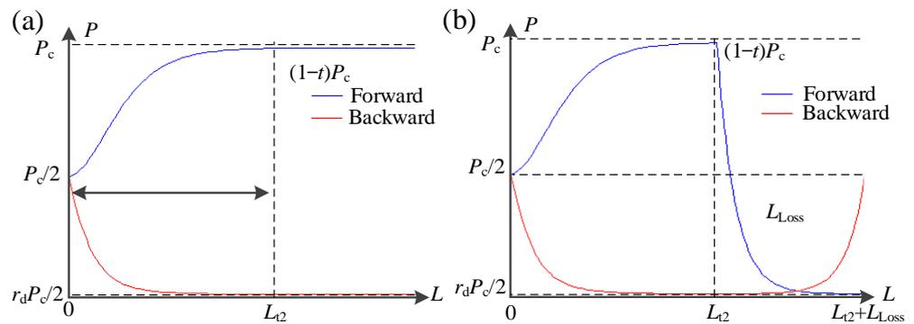
**Figure 5.** Simulated results of propagation properties of (a) the saturated gain waveguide and (b) connecting a linear loss waveguide in the isolator working at duplex mode.
