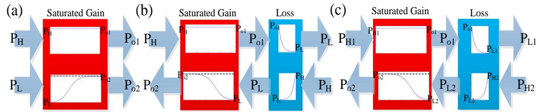
**Figure 3.** (a) Saturated gain property, (b) schematic diagram of simplex operating mode and (c) duplex operating mode.  $P_H \gg P_L, P_{o1} \approx P_{o2} \approx P_H \approx P_c$ .
