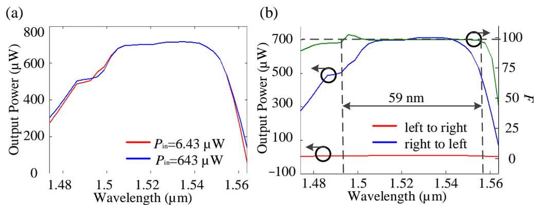
**Figure 9.** (a) Simulated broadband transmission characteristic of the SOA. (b) Simulated broadband transmission and isolating factor of the whole device.
