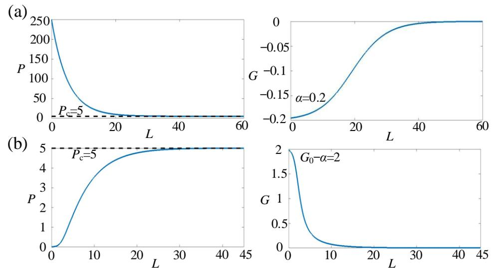
**Figure 2.** Blue line: Theoretical curves of functions  $P(L)$  and  $G(L)$  when the input power is (a) lower and (b) higher than  $P_c$ . Dotted:  $P_c = 5$ .
