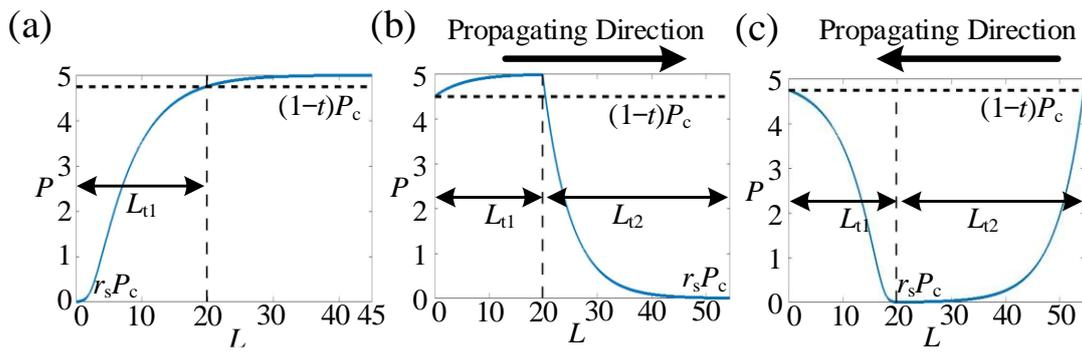
**Figure 4.** Blue line: Simulated results of propagation properties of the saturated gain waveguide (a), the proposed isolator when signals transmit forward (b) and backward (c).
