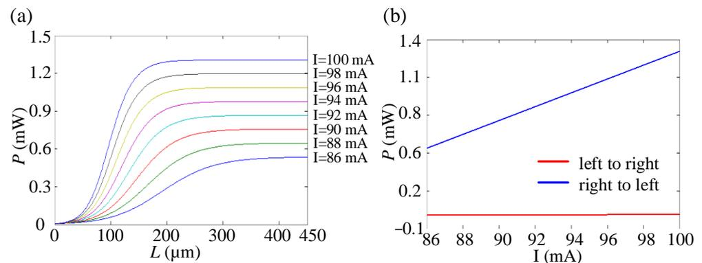
**Figure 10.** (a)  $P$ - $L$  curves of the SOA with different pump currents. (b) Operation power of the isolator with different pump currents. All the curves are simulated using FDTD.
