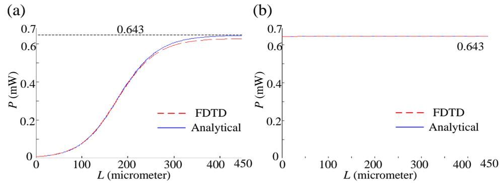
**Figure 7.** FDTD-simulated and analytical results of relation between  $P$  and  $L$  when a signal with (a)  $6.43 \mu\text{W}$  and (b)  $643 \mu\text{W}$  inputs power. Black dotted lines:  $P = 0.643$ .
