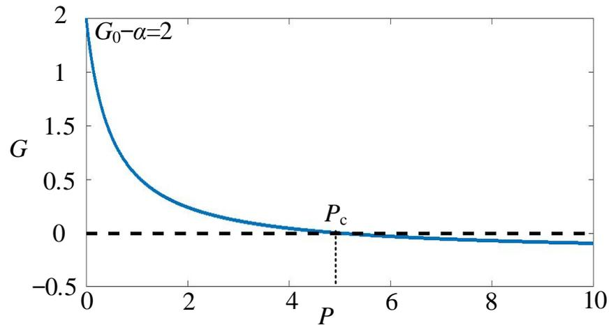
**Figure 1.** Blue line: Relation between the gain coefficient  $G$  and light power  $P$ .  $P_c$  is the cut-off power. Parameters of this case. The result is simulated with  $G_0 = 2.2$ ,  $P_s = 0.5$ , and  $\alpha = 0.2$ . Dotted:  $G = 0$ .
