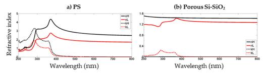
**Figure 3.** Theoretical values of the complex refractive index for PS and porous Si-SiO<sub>2</sub> layers. (a) The complex refractive index values for PS layers and (b) for porous Si-SiO<sub>2</sub> layers obtained from both models.
