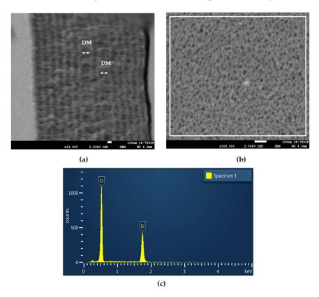
**Figure 5.** (a) Cross-section SEM of an oxidized PQS on a quartz substrate with 30 layers. (b) SEM image of the superficial section of an oxidized PQS on a quartz substrate. The SEM images show two defect layers (white arrows) between two BRs. The layers with low porosity can be observed in light gray, and layers with high porosity are displayed in dark gray. (c) EDS elemental spectrum, the white rectangle on (b) displays the selected area taken to obtain the EDS measurements.
