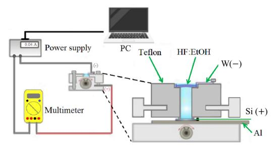
Figure 1. The electrochemical etching setup and the various parts of the etching cell.
