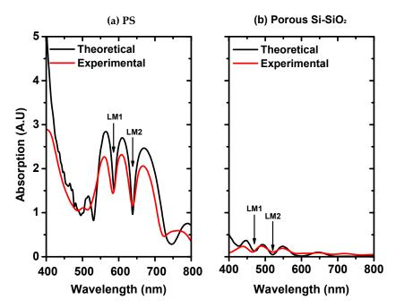
**Figure 6.** Theoretical and experimental absorption spectra comparison for a PQS made of PS and porous Si-SiO<sub>2</sub>. (a) Theoretical (black line) and experimental (red line) absorption spectra of a PS PQS and (b) theoretical (black line) and experimental (red line) absorption spectra of a porous Si-SiO<sub>2</sub> PQS.
