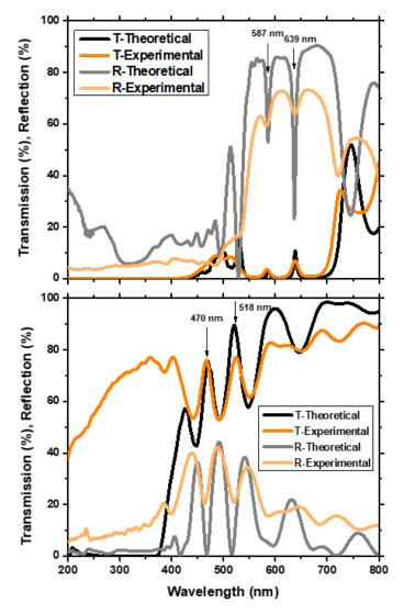
**Figure 4.** Theoretical and experimental reflection and transmission spectra of unoxidized and oxidized periodic/quasiperiodic structures. **(Top)** Theoretical and experimental reflection and transmission spectra of unoxidized periodic/quasiperiodic structure. **(Bottom)** Theoretical and experimental reflection and transmission spectra of oxidized periodic/quasiperiodic structures.
