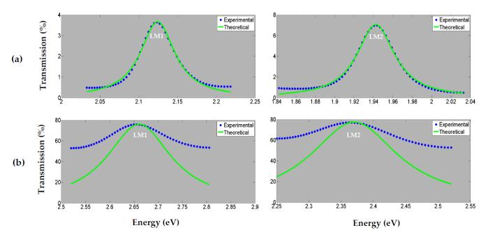
**Figure 7.** Comparison of the experimental transmission spectrum (blue line) with the theoretical transmission calculated using the Breit–Wigner's equation modified by Miller (green line) for two LM before (a) and after (b) dry oxidation.
