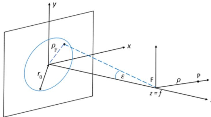
**Figure 3.** Schematic diagram with notations for the study of focusing radially polarized wave with a focusing element (the blue circle in the x-y plane) having small numerical aperture. The observation point P is located at a distance  $\rho$  from the z axis. The dashed line is a ‘ray’ passing through the focus F.
