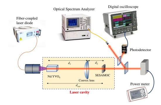
**Figure 1.** Experimental setup of passively mode-locked solid-state laser for exploring the buildup dynamics in the turn-on process.
