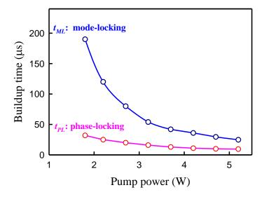
**Figure 6.** Experimental results for the buildup times for the complete phase locking and stable mode locking versus the pump power.
