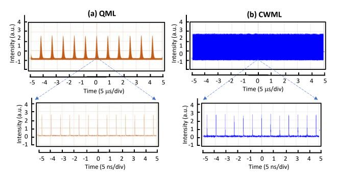
**Figure 2.** Measured oscilloscope traces at two different time spans for (**a**) the operation of QML obtained at the pump power of 1.0 W and (**b**) the operation of CWML obtained at the pump power of 2.0 W.
