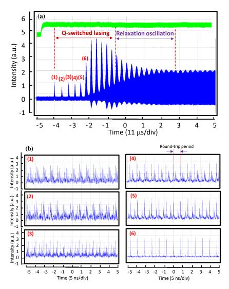
**Figure 5.** (a) Oscilloscope traces for the transient dynamics measured at a pump power of 2.6 W in a time span of 55  $\mu$ s; green lines: pump light; blue lines: laser output. (b) Temporal traces in a time span of 50 ns measured from the intensities inside the first six Q-switched envelopes shown in (a).
