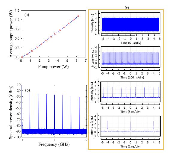
**Figure 3.** (a) Average output power versus the pump power for the laser operation. (b) Measured power spectral density at a pump power of 3.0 W for a representative case of the experimental results. (c) Measured oscilloscope traces at four different time spans ranging from 10 ns to 50 µs.
