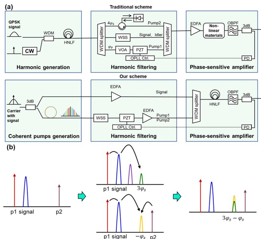
**Figure 1.** (a) Comparison between traditional scheme and ours; (b) the principle of single-step phase-sensitive regeneration of QPSK. CW: Continuous wave laser; WDM: wavelength-division multiplexer; HNLF: highly non-linear fibers; WSS: wavelength selective switch; VOA: variable optical attenuator; PZT: piezoelectric transducer; OPLL: optical phase-locked loop; OBPF: 0.8 nm optical bandpass filter; 3 dB: 3 dB splitter; EDFA: erbium-doped fiber amplifier; PD: photodetector.
