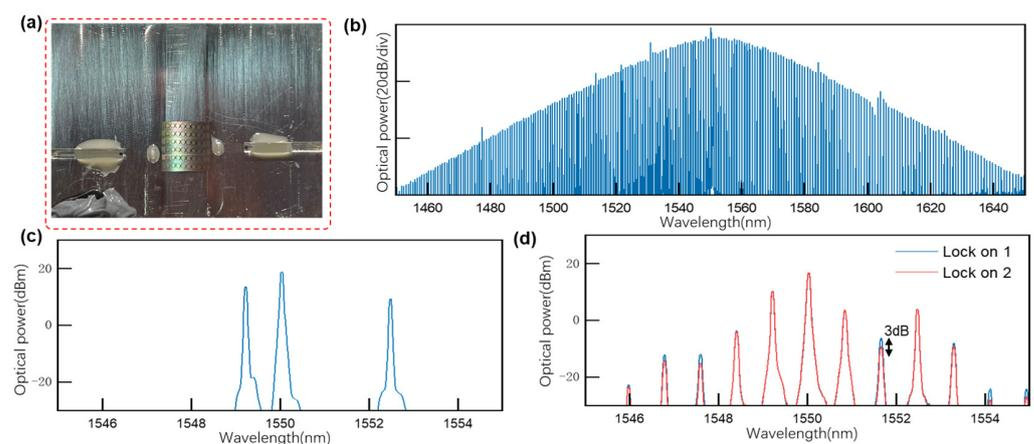
**Figure 3.** (a) The pictures of packaged Si<sub>3</sub>N<sub>4</sub> chips used in our experiment. (b) Measured optical spectrum for Kerr soliton comb, which is generated in the part of coherent pump generation. (c) The input spectrum of the HNLF. (d) Output spectrum under conditions that satisfy different phase matching between the signal and the pump. The regeneration signal experiences a phase jitter of 3 dB at the idle frequency.
