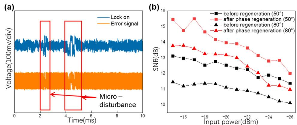
**Figure 5.** (a) Servo output signal (blue) and error signal (yellow); (b) shows the calculated SNR before (black) and after regeneration (red).
