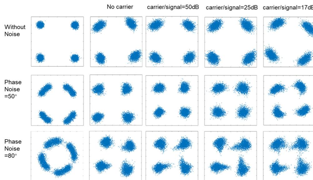
**Figure 4.** Constellation diagrams of different input carrier ratios with no noise, 50 degrees of phase noise, and 80 degrees of phase noise.
