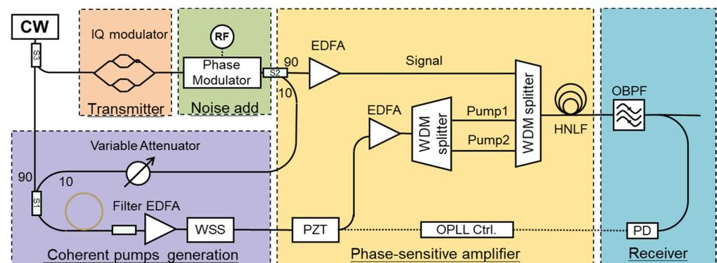
**Figure 2.** The experimental setup of single-step phase-sensitive regeneration of QPSK. RF: Radio Frequency; S1 and S2: 10:90 optical splitter; S3: 3 dB splitter.
