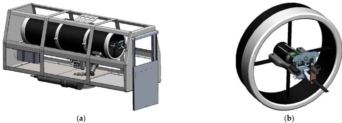
Figure 3. CAD image of the (a) instruments internal configuration and (b) laser diode collimator mount.
