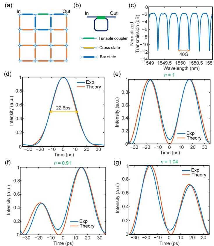
**Figure 5.** Experimental results for Hilbert transformation. (a) Waveguide mesh configuration diagram. (b) Mesh connection layout. (c) Measured transfer function of the reconfigured MRR. (d) The input Gaussian pulse with a temporal width of 22.6 ps. (e–g) The calculated (orange curve) and measured (blue curve) fractional differentiation of the input Gaussian pulse with fraction orders of 1 (e), 0.91 (f), and 1.04 (g).
