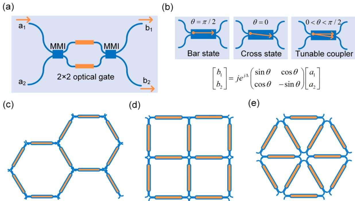
**Figure 1.** Universal  $2 \times 2$  optical gate. (a) The magnitude and phase of output light  $b_1$  and  $b_2$  are controlled through the  $2 \times 2$  optical gate. (b) The gate can be tuned in bar, cross, and tunable coupler states. (c–e) Reconfigurable waveguide meshes based on a hexagonal topology (c), quadrilateral topology (d), and triangular topology (e).
