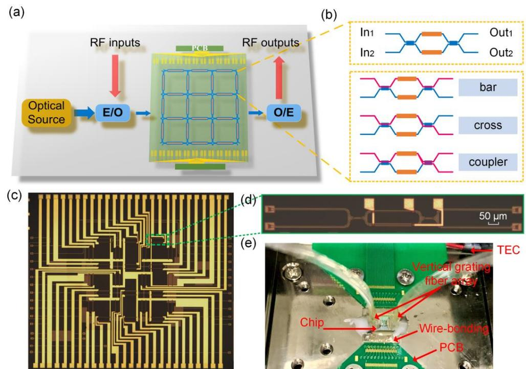
**Figure 2.** Schematic of the proposed programmable photonic integrated computing chip. (a) Reconfigurable hardware core and the possible electrical and optical peripherals. (b) Schematic representation of the basic MZI unit. (c) Microscope image of the fabricated photonic computing chip. (d) Zoomed-in image of a basic optical gate. (e) Overall photo of the packaged chip with TEC temperature control.
