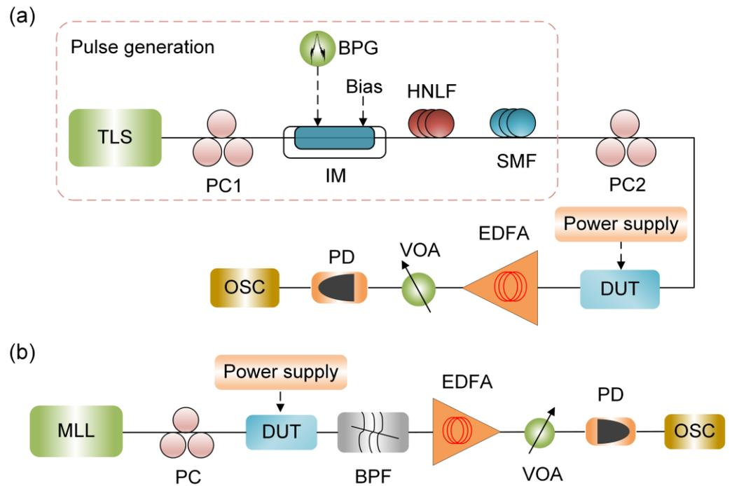
**Figure 3.** Experimental setup for temporal differentiation, Hilbert transformation (a), and temporal integration (b). TLS, tunable laser source; PC, polarization controller; BPG, bit pattern generator; IM, intensity modulator; HNLF, high nonlinear fiber; SMF, single-mode fiber; DUT, device under test; EDFA, erbium-doped fiber amplifier; VOA, variable optical attenuator; PD, photodetector; OSC, oscilloscope; MLL, mode-locked laser; BPF, bandpass filter.
