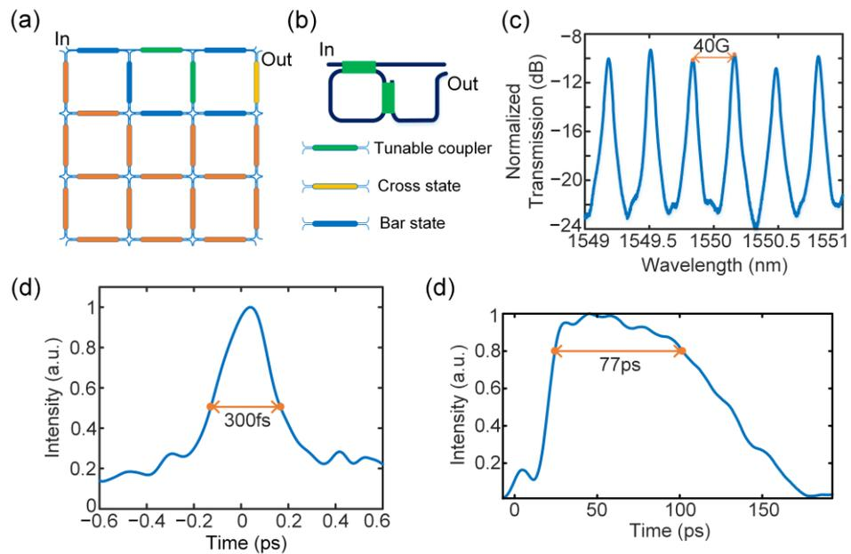
**Figure 6.** Experimental results for temporal integration. (a) Waveguide mesh configuration diagram. (b) Mesh connection layout. (c) Measured transfer function of the reconfigured add–drop MRR. (d) The input Gaussian pulse with a temporal width of 300 fs. (e) The integration of the Gaussian pulse with an integration time of 77 ps.
