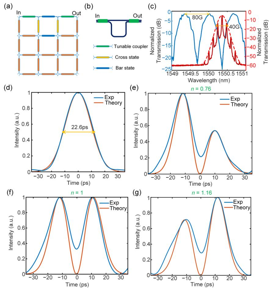
**Figure 4.** Experimental results for fractional differentiation. (a) Waveguide mesh configuration diagram. (b) Mesh connection layout. (c) Measured transfer function of the reconfigured MZI (blue curve) and the optical spectrum of the Gaussian input (red curve). (d) The input Gaussian pulse with a temporal width of 22.6 ps. (e–g) The calculated (orange curve) and measured (blue curve) fractional differentiation of the input Gaussian pulse with fraction orders of 0.76 (e), 1 (f), and 1.16 (g).
