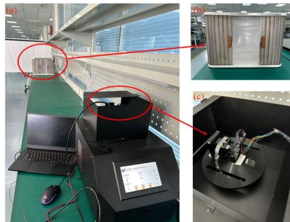
Figure 7. (a) Responsiveness experimental test system. (b) Air box with controllable air bag width. (c) Rotating platform of the responsiveness test system.
