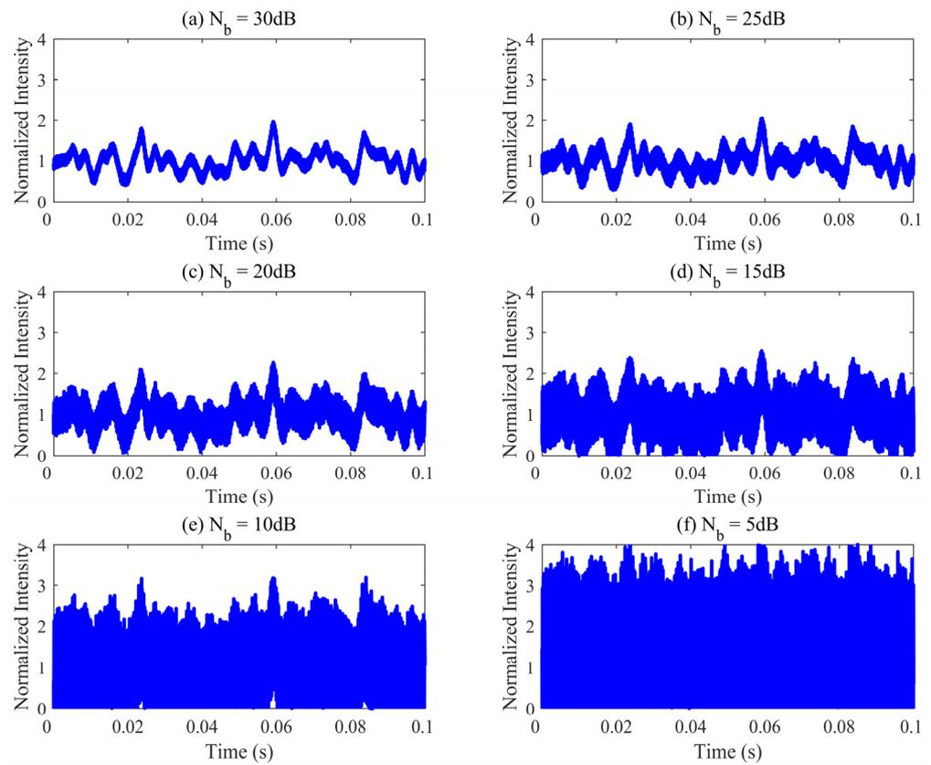
**Figure 6.** Time-domain performance of a signal through the turbulent channel of  $\sigma^2 = 0.0596$  with different background noises. (a)  $N_b = 30$  dB, (b)  $N_b = 25$  dB, (c)  $N_b = 20$  dB, (d)  $N_b = 15$  dB, (e)  $N_b = 10$  dB, (f)  $N_b = 5$  dB.
