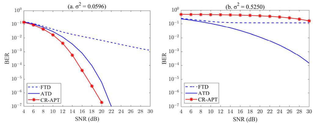
**Figure 8.** BER performance of the three techniques in different turbulent channels when  $N_b = 25$  dB. (a)  $\sigma^2 = 0.0596$ , (b)  $\sigma^2 = 0.5250$ .
