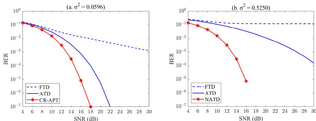
**Figure 5.** Ideal BER performance of the three techniques in two channels with different turbulence strengths. (a)  $\sigma^2 = 0.0596$ , (b)  $\sigma^2 = 0.5250$ .
