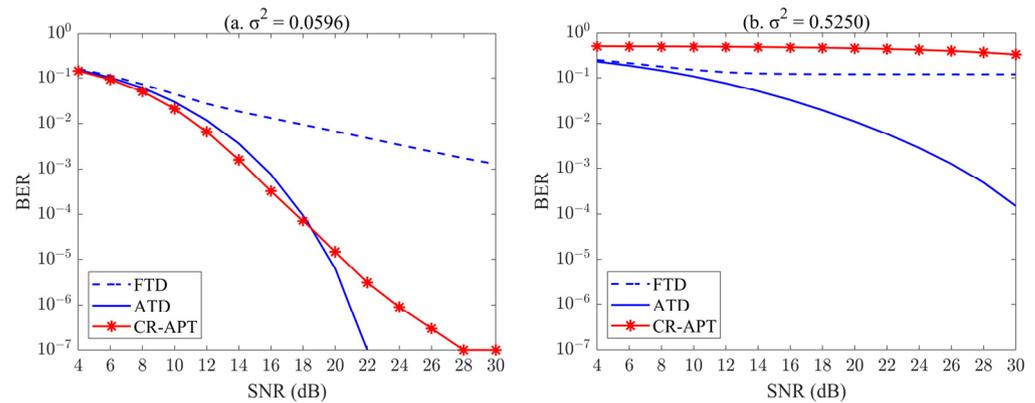
**Figure 9.** BER performance of the three techniques in different turbulent channels when  $N_b = 20$  dB. (a)  $\sigma^2 = 0.0596$ , (b)  $\sigma^2 = 0.5250$ .
