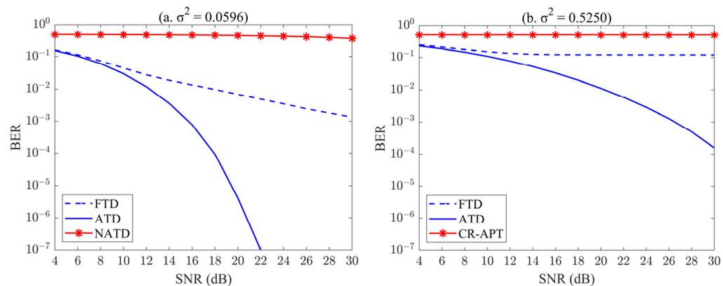
**Figure 11.** BER performance of the three techniques in different turbulent channels when  $N_b = 10$  dB. (a)  $\sigma^2 = 0.0596$ , (b)  $\sigma^2 = 0.5250$ .
