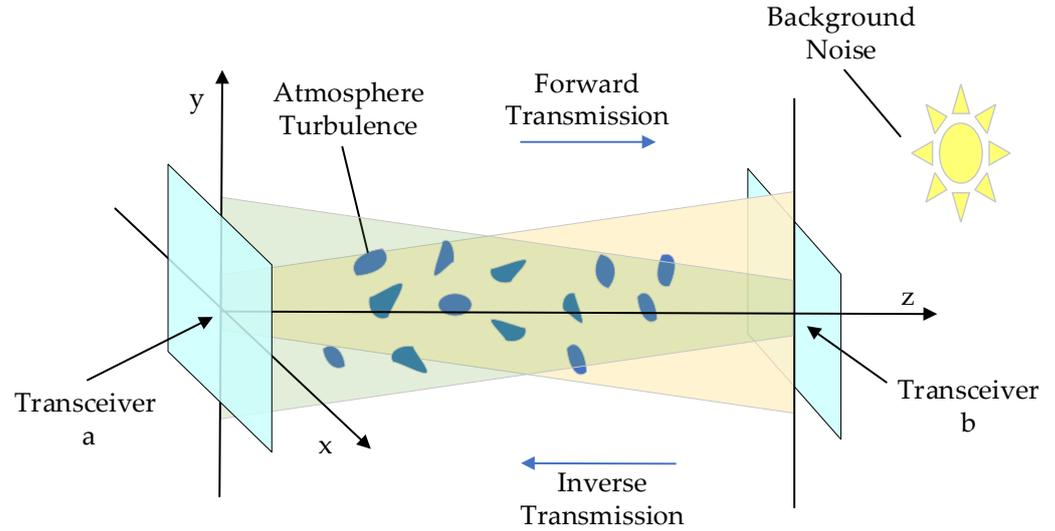
Figure 1. Schematic of bidirectional atmospheric channel model.
