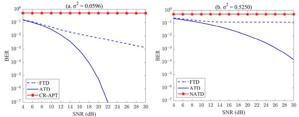
**Figure 12.** BER performance of the three techniques in different turbulent channels when  $N_b = 5$  dB. (a)  $\sigma^2 = 0.0596$ , (b)  $\sigma^2 = 0.5250$ .
