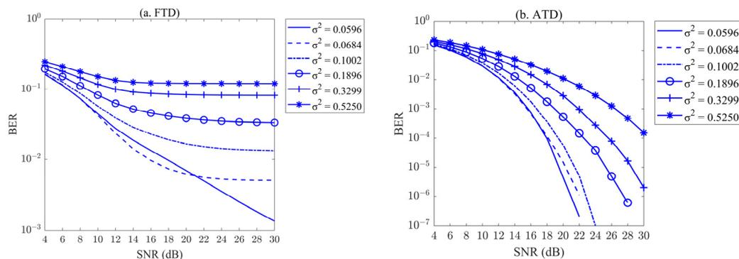
**Figure 3.** (a) Performance of FTD in different turbulent channels. (b) Performance of ATD in different turbulent channels.
