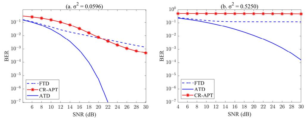
**Figure 10.** BER performance of the three techniques in different turbulent channels when  $N_b = 15$  dB. (a)  $\sigma^2 = 0.0596$ , (b)  $\sigma^2 = 0.5250$ .
