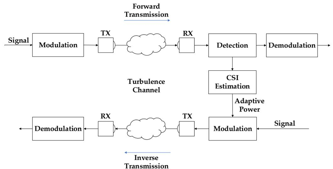
Figure 2. Block diagram of adaptive power transfer system.
