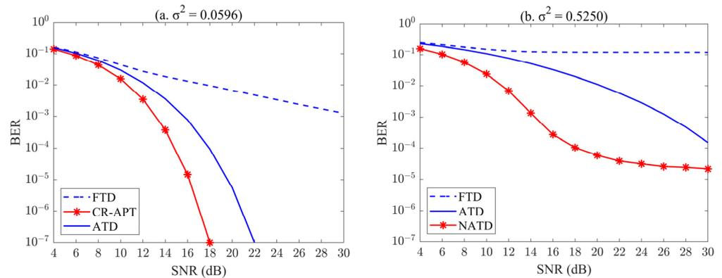
**Figure 7.** BER performance of the three techniques in different turbulent channels when  $N_b = 30$  dB. (a)  $\sigma^2 = 0.0596$ , (b)  $\sigma^2 = 0.5250$ .
