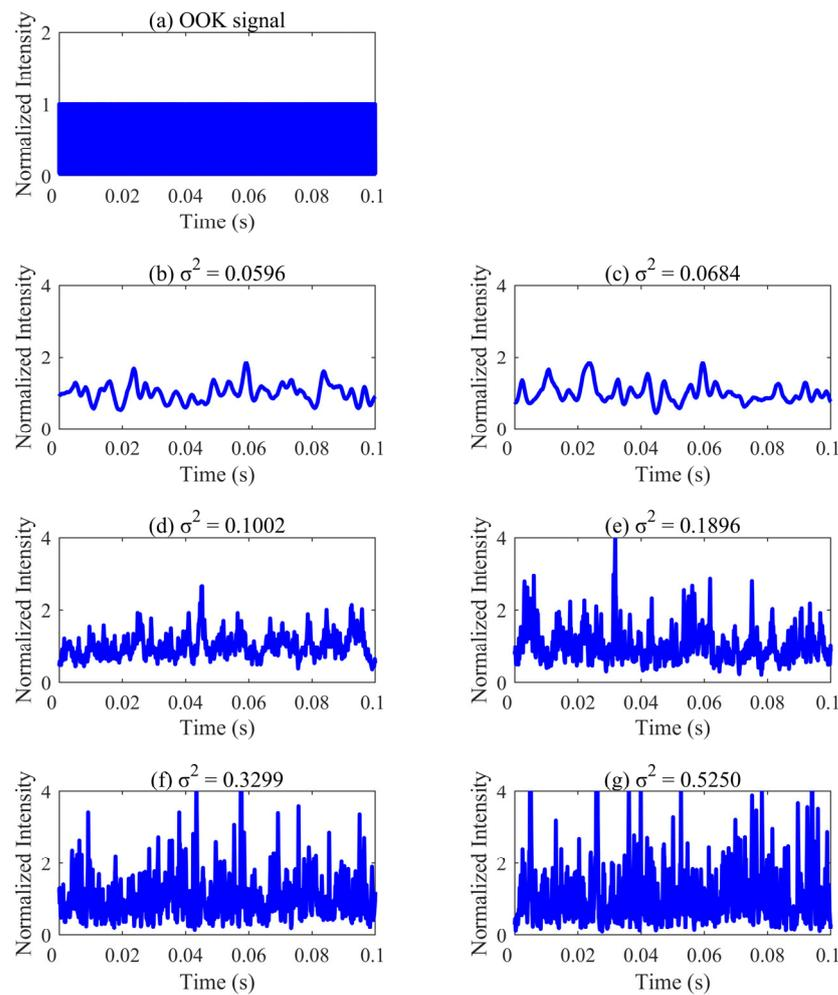
**Figure 4.** Plot of the time-domain performance of the signal as it passes through different turbulent channels;  $\sigma^2$  represents channel turbulence intensity. (a) OOK signal, (b)  $\sigma^2 = 0.0596$ , (c)  $\sigma^2 = 0.0684$ , (d)  $\sigma^2 = 0.1002$ , (e)  $\sigma^2 = 0.1896$ , (f)  $\sigma^2 = 0.3299$ , (g)  $\sigma^2 = 0.5250$ .
