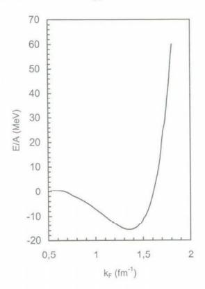
**Figure I.** Binding energy per nucleon for the nuclear matter as a function of density.
