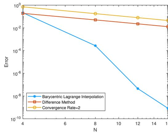
Figure 1. Spatial  $L^\infty$  errors at  $t = 1$  for NLS equation for Example 1.
