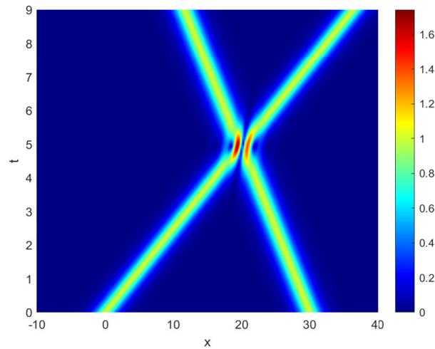
Figure 4. The interaction of two solitary waves without damping at  $T = 9$  for Example 2.
