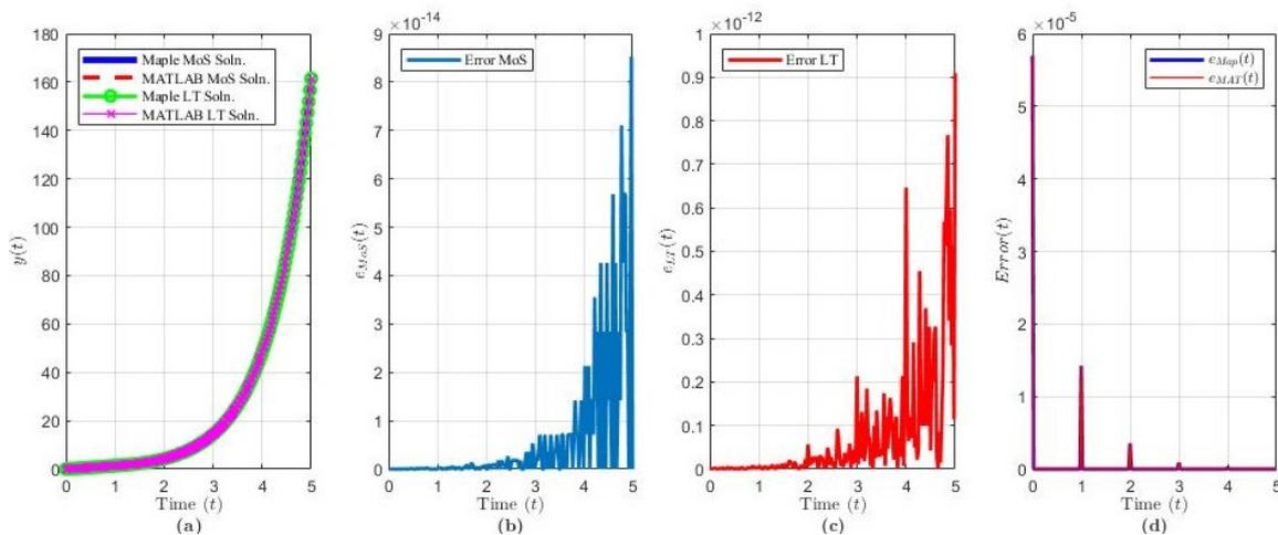
**Figure 4.** Solution results of Equation (21) over  $t \in [0, 5\tau]$  ( $n = 2000$  terms): plot of (a) the solution  $y(t)$  via each method and software, (b)  $e_{MoS}(t)$ , (c)  $e_{LT}(t)$ , (d)  $e_{Map}(t)$  and  $e_{MAT}(t)$ .
