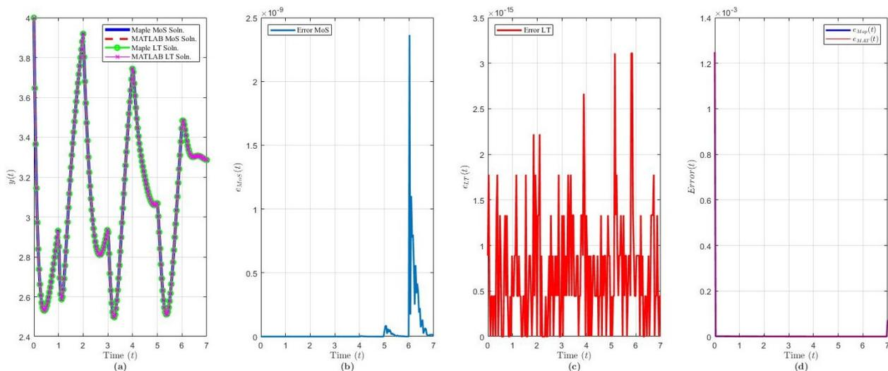
**Figure 8.** Solution results of Equation (25) over  $t \in [0, 7\tau]$  ( $n = 500$  terms): plot of (a) the solution  $y(t)$  via each method and software, (b)  $e_{MoS}(t)$ , (c)  $e_{LT}(t)$ , (d)  $e_{Map}(t)$  and  $e_{MAT}(t)$ .
