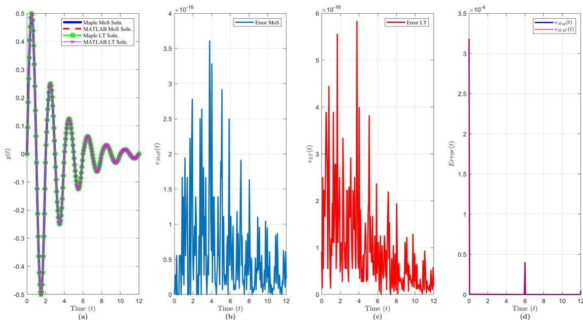
**Figure 5.** Solution results of Equation (22) over  $t \in [0, 6\tau]$  ( $n = 500$  terms): plot of (a) the solution  $y(t)$  via each method and software, (b)  $e_{MoS}(t)$ , (c)  $e_{LT}(t)$ , (d)  $e_{Map}(t)$  and  $e_{MAT}(t)$ .
