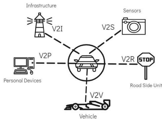
**Figure 3.** Epic wireless communication with the internet of vehicles.
