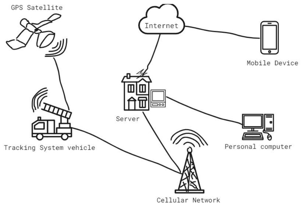
**Figure 5.** Real-time GPS tracker system.
