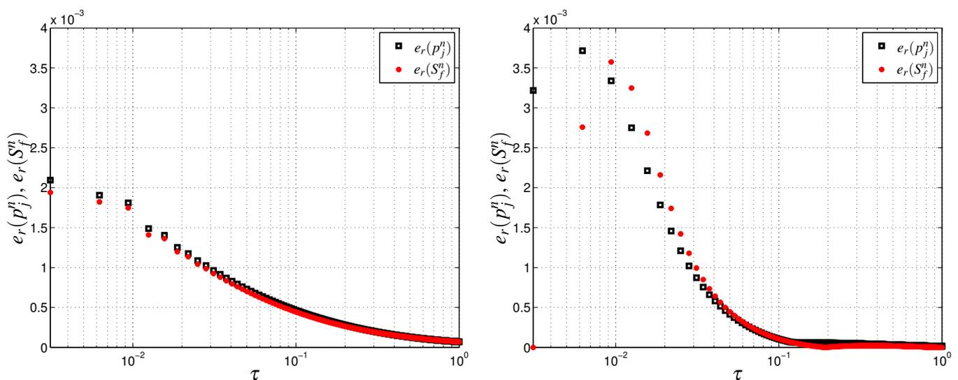
**Figure 6.** Numerical estimated errors  $e_r(p^n)$  and  $e_r(S_f^n)$  versus  $\tau^n$  for the explicit (left) and implicit method (right), setting  $\epsilon = 0.005$ ,  $\mu = 20$ ,  $J_5 = 160$  and  $N_5 = 1280$ .
