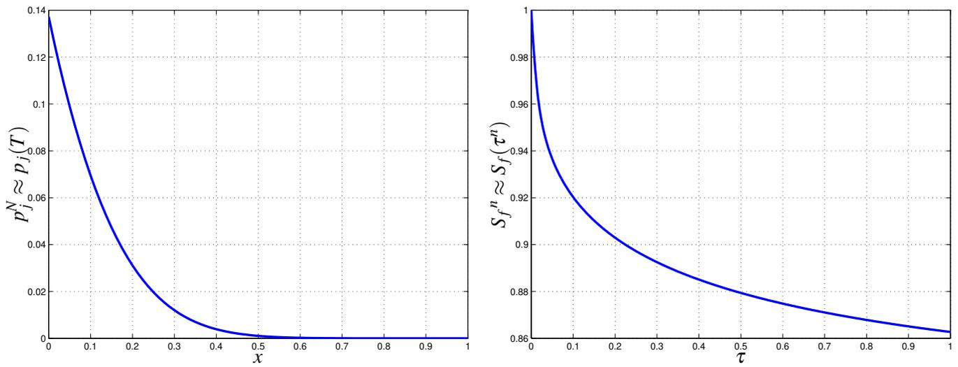
**Figure 4.** Numerical results obtained by the implicit scheme (8): on the left  $p_j^N$  versus  $x_j$ , on the right,  $S_f^n$  versus  $\tau^n$ , obtained with  $J = 80$ ,  $N = 320$  and  $\mu = 20$ .
